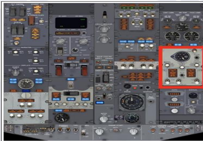
Figura 6 - Boeing 737NG Overhead Panel. Fonte: Flight Crew Operations Manual (FCOM).
