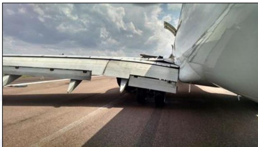
Figura 35 - Danos na asa da aeronave VT-JGA após a quebra do aft trunnion pin . Fonte: Final Investigation Report on Accident to M/s Jet Airways (Pvt.) Ltd. Boeing B 737-800 Aircraft VT-JGA at Khajuraho Airport.
