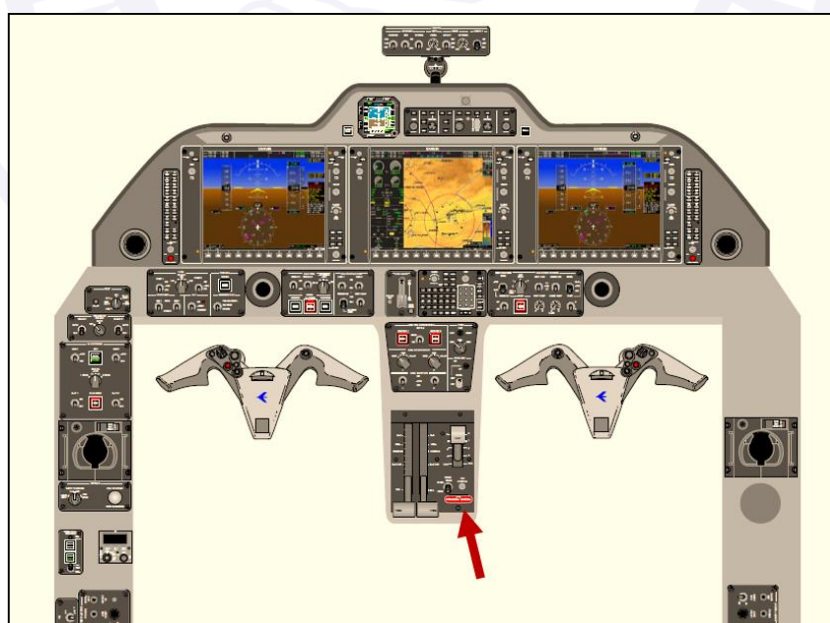
Figura 6 - Alavanca do EPB - Main/Glareshield/Control Pedestal Panels. Fonte: Phenom 300 Pilot's Operating Handbook .
