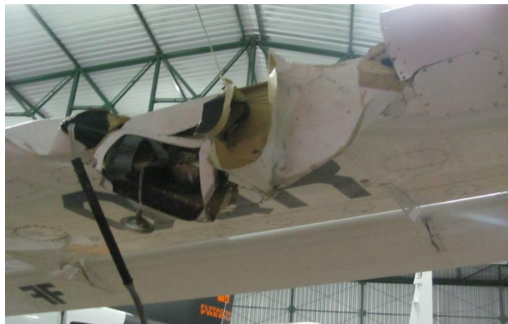
Figure 6 – Wing damage, as observed during the initial action.
