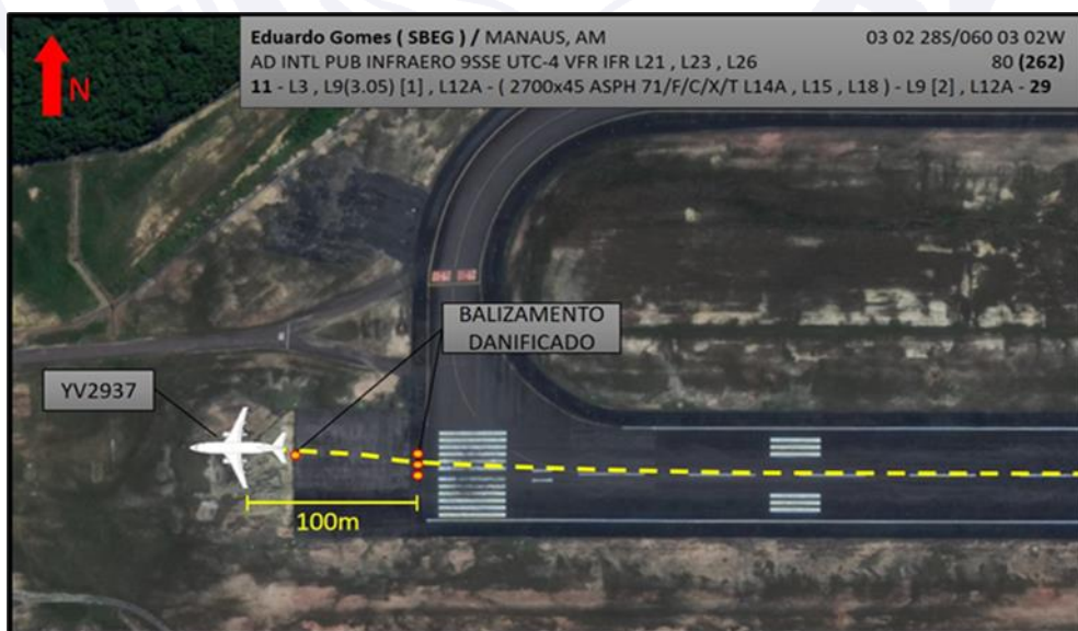
Figure 6 - Sketch with the final position of the aircraft and damage caused to the SBEG runway marking.
