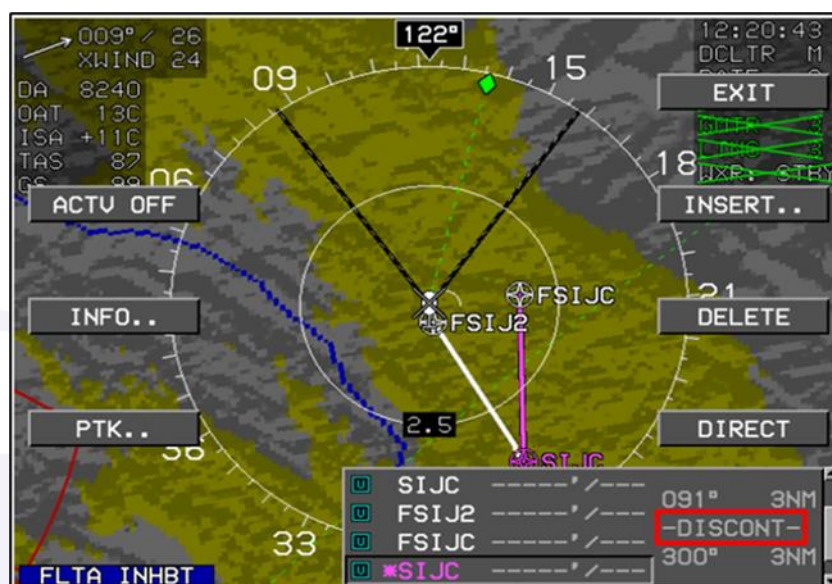
Figure 24 - Simulated HSI with flight plan overlay in MAP format.
