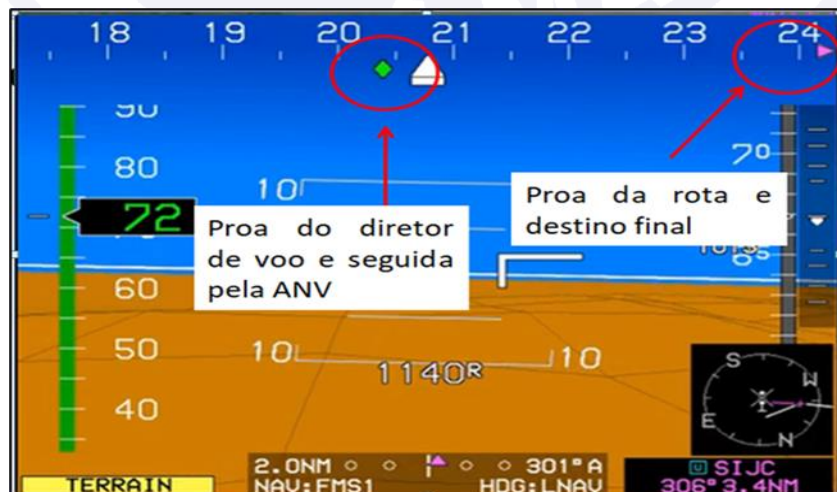
Figure 29 - Reconstruction of the ADI view.
