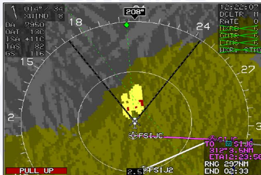
Figure 15 - Reproduction of the HSI indications (in MAP format) during the final descent.
