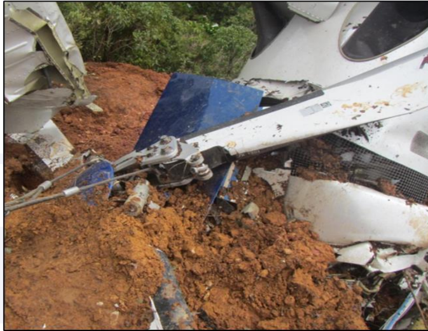
Figure 12 – Detail of the upper frontal section burying, highlighting one of the main rotor blades.
