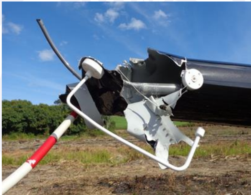
Figure 2 - View of the sectioned tail cone.
