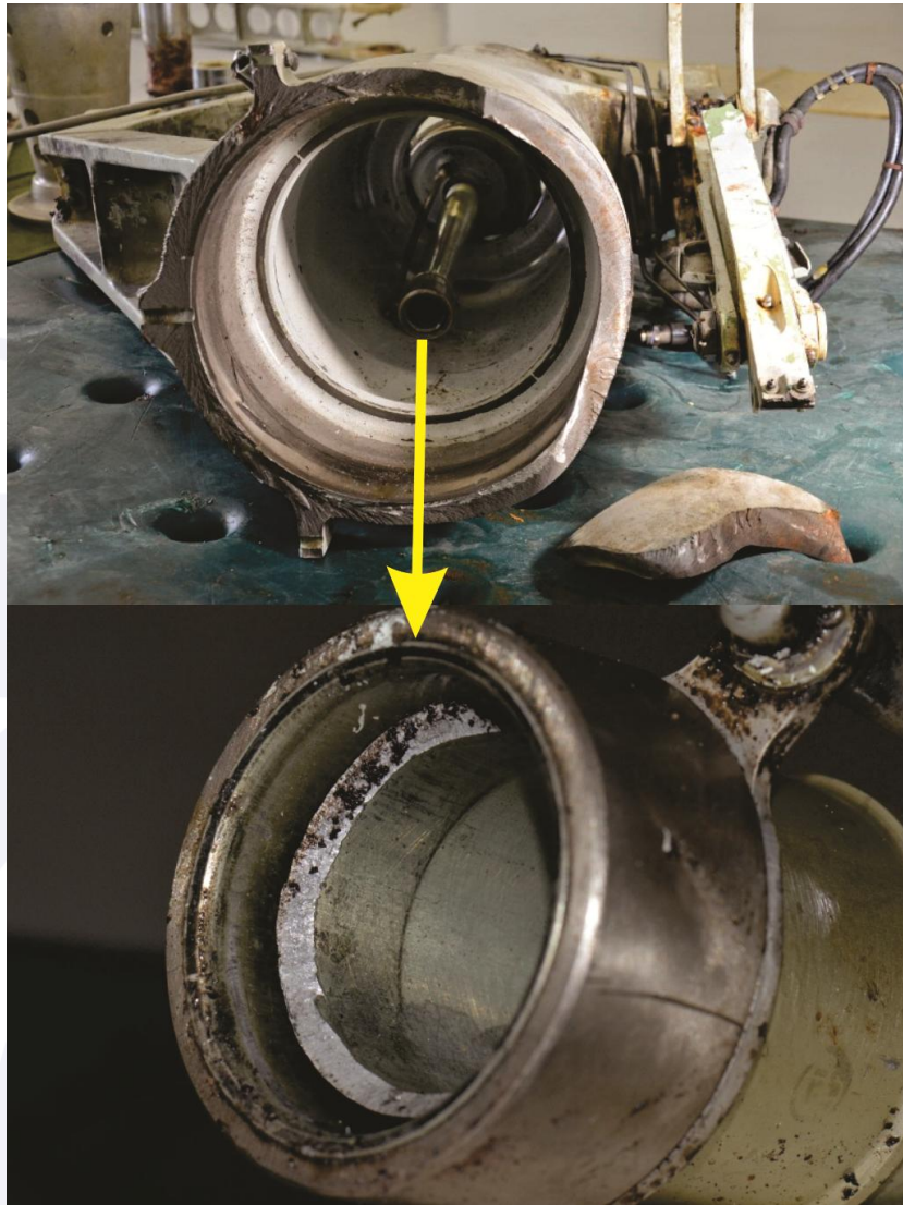
Figure 4 – General view of the cylinder interior and a fracture with a 45-degree incline in the interior of the tube (typical fracture due to overload).
