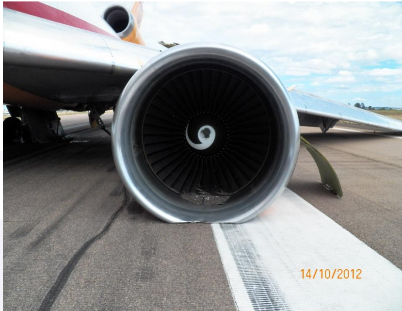
Figure 1 – Position of the aircraft on the runway, showing the damage to the left main gear, left wing and left engine.
