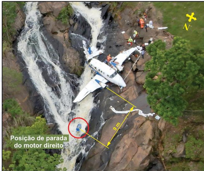
Figure 18 - Identification of the stop location for the right engine/propeller.
