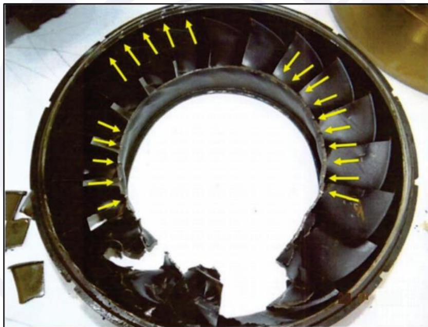
Figure 31 - Rear view of the left engine power turbine stator with stopped impact marks and damage to the fins.
