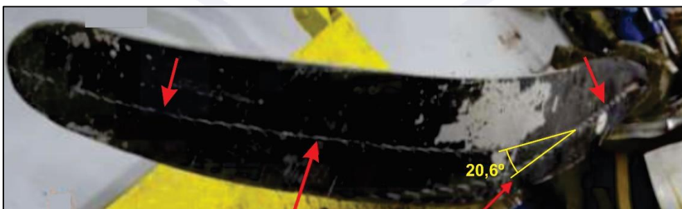
Figure 41 - Details of the impact marks of the cable against the left engine propeller blade.
