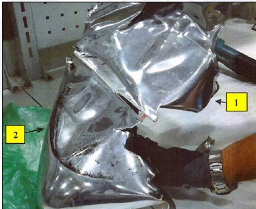
Figure 33 - Impact marks on the left engine spinner.
