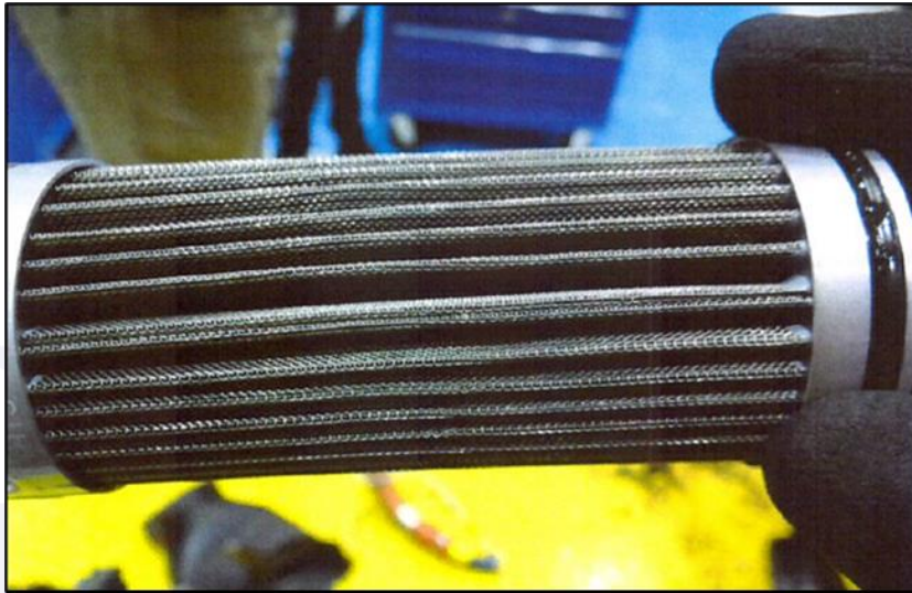
Figure 32 - Left engine oil filter without abnormalities.
