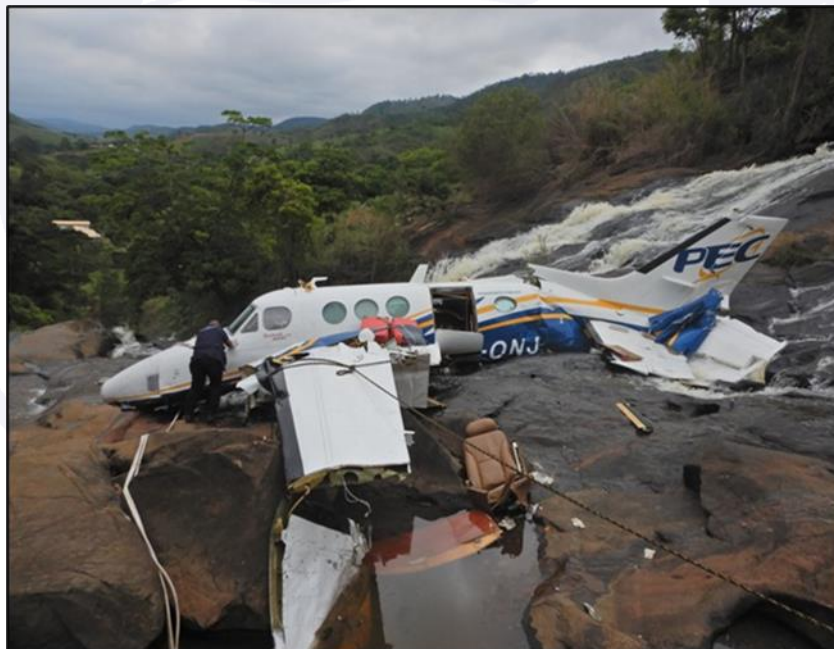
Figure 19 - Location of the final stop and damage to the aircraft structure.
