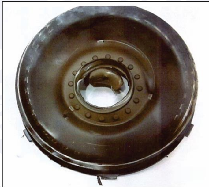
Figure 29 - Rear view of the diaphragm with smooth rubbing and impact marks with the power turbine rotor stopped.
