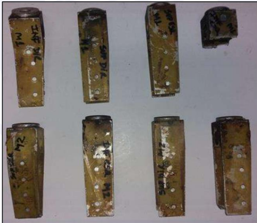
Figure 43 - (A) Engine fixing brackets of the left engine (above) and the right engine (below).
