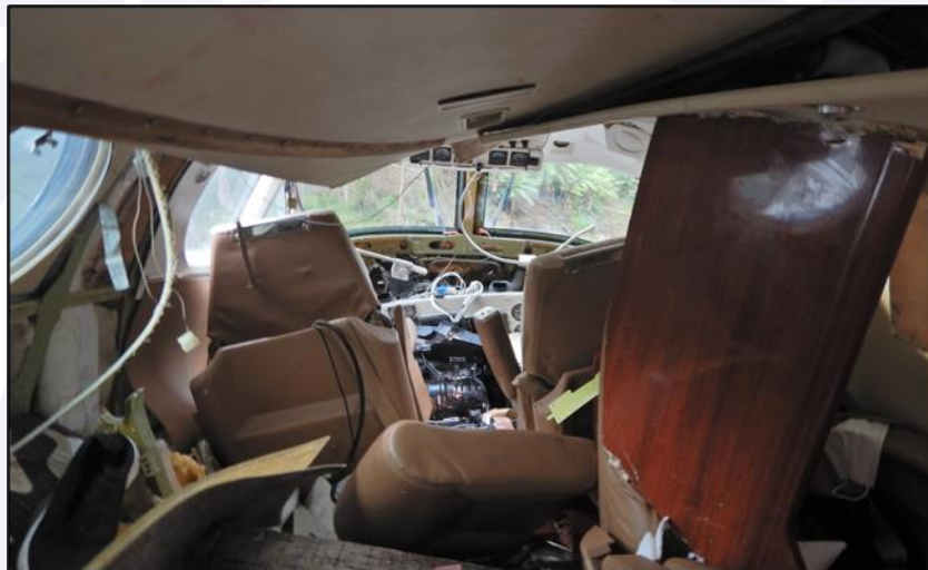
Figure 22 - Extent of damage inside the aircraft.
