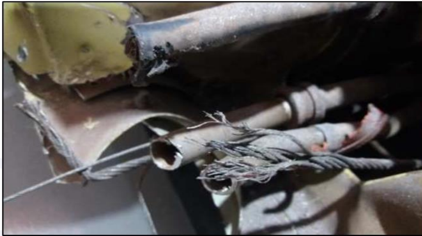
Figure 23 - Aircraft control cables with overload indicator.
