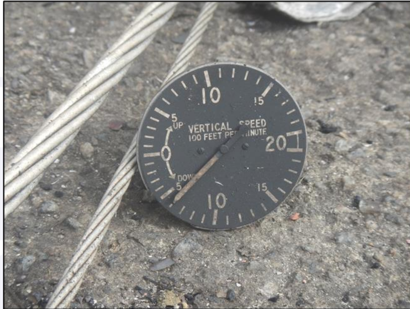
Figure 4 - Vertical Speed Indicator (Climb) showing a descent rate of 600 ft/min.
