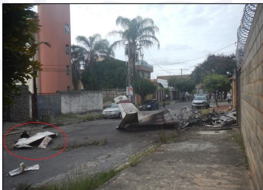
Figure 3 - Image of the accident site. In the red highlight, the part of the left-wing that separated from the plane.
