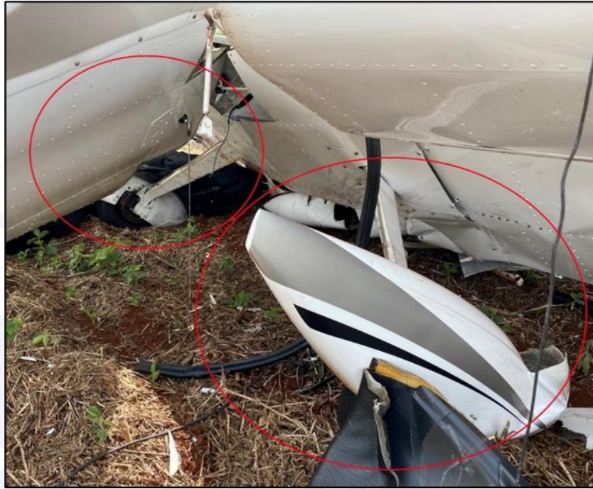
Figure 7 - Condition of the main landing gears after impact.
