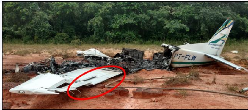
Figure 5 - Approximate view of the aircraft. In detail, it shows that the flaps were retracted.
