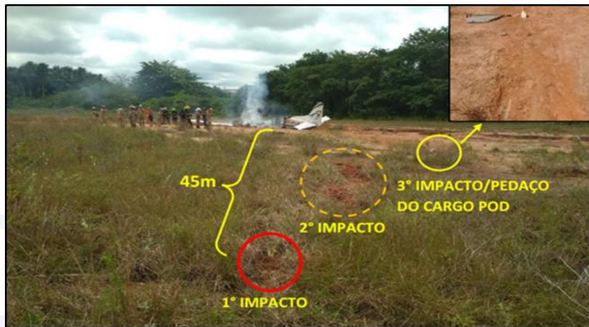
Figure 4 - General view of the wreckage. The red circle indicates the point of the 1 st impact, the dashed orange circle indicates the 2 nd impact and the yellow circle shows the 3 rd impact (part of the Cargo Pod in the detail).
