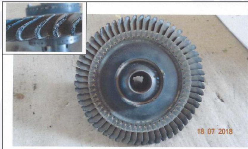
Figure 8 - Images of the compressor turbine rotor. The highlight shows a superior view of the top of the vanes, where part of the material has been melted.
