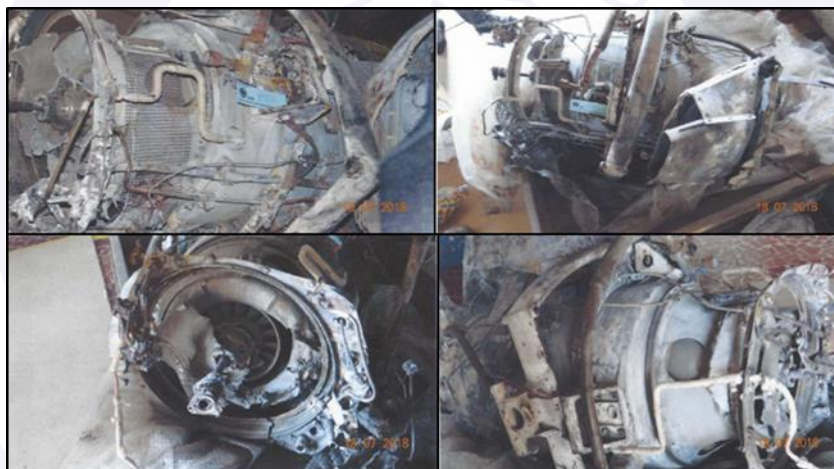
Figure 6 - Images of the engine, in which the damage to the sides and rear resulting from the action of fire is observed.
