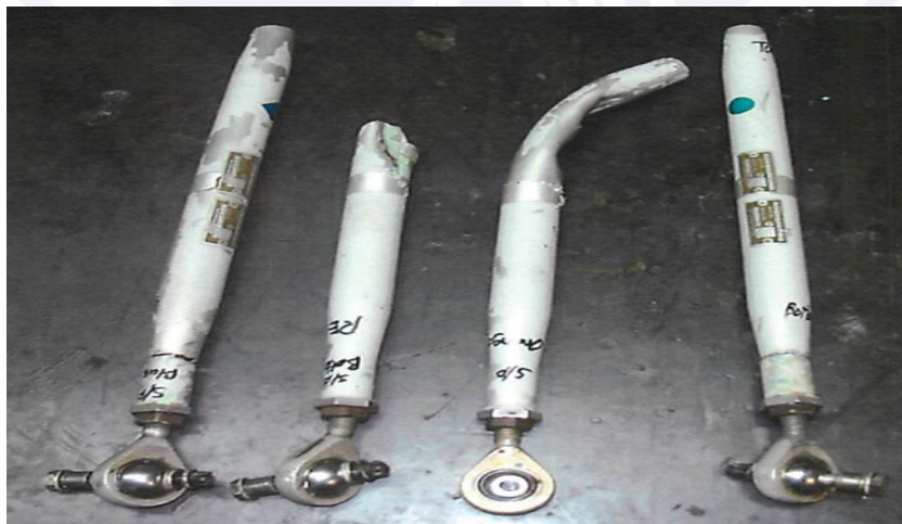
Figure 3 - Main rotor blade links. Deformation fractures caused by overload.
