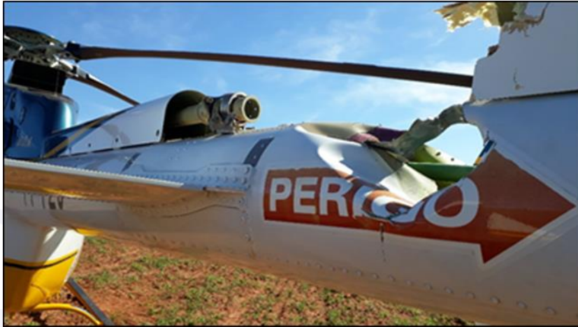
Figure 7 - Detail of the point of impact of the main rotor blades against the tail boom.
