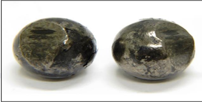
Figure 21 - View of the damage caused to the spheres of bearing nº 2.
