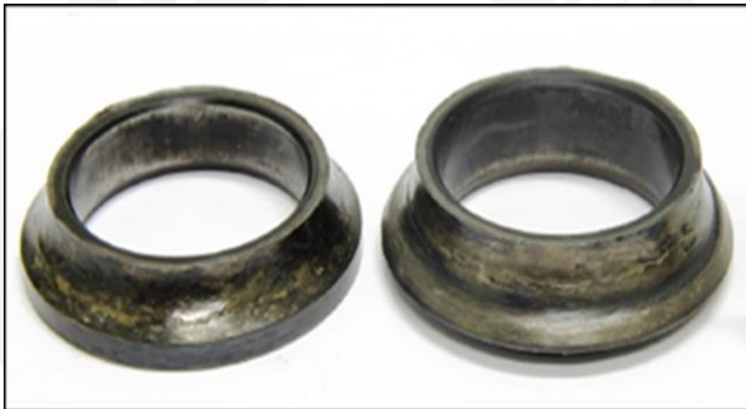
Figure 19 - View of the general condition of the inner rings of bearing n° 2.
