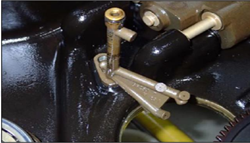
Figure 15 - Piccolo tube in its correct position.
