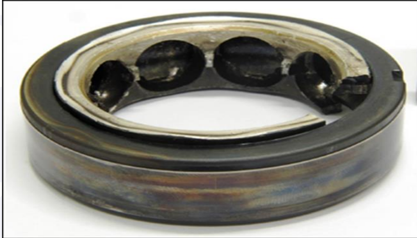
Figure 18 - General view of bearing n°2 and damage to its rail.
