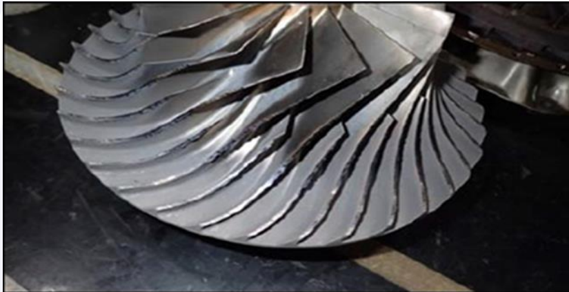
Figure 13 - View of the compressor axial stage.
