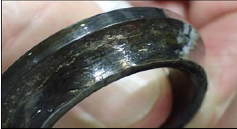
Figure 12 - Scratch marks on the inner raceway of bearing n°2.
