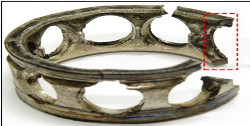
Figure 22 - View of the inner rails of bearing nº 2.
