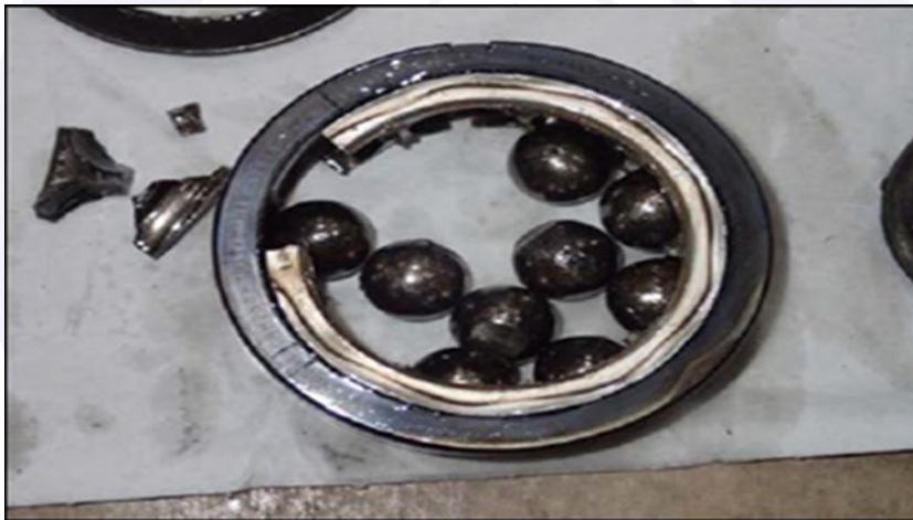
Figure 10 - Bearing n° 2 after being removed from the aircraft.
