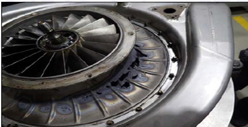
Figure 14 - Damage to the compressor area.
