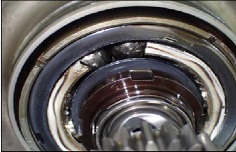
Figure 9 - Bearing n° 2 in its correct position, but damaged.
