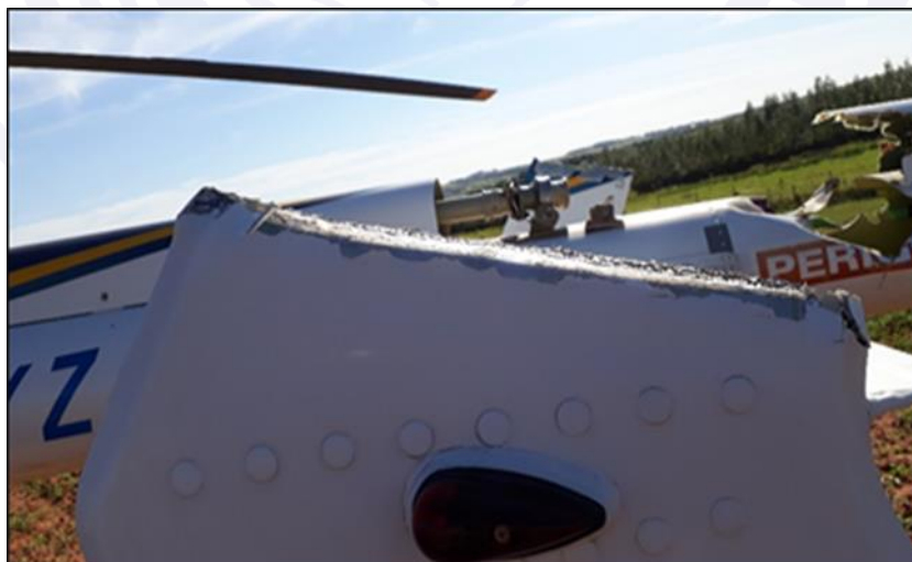
Figure 6 - Detail of the left finlet cutting angle caused by the main rotor.
