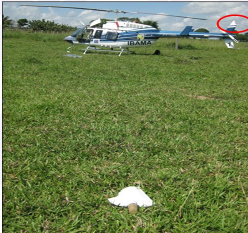
Figure 4 - Overview. On the detail, the piece of the vertical stabilizer sectioned after the collision.
