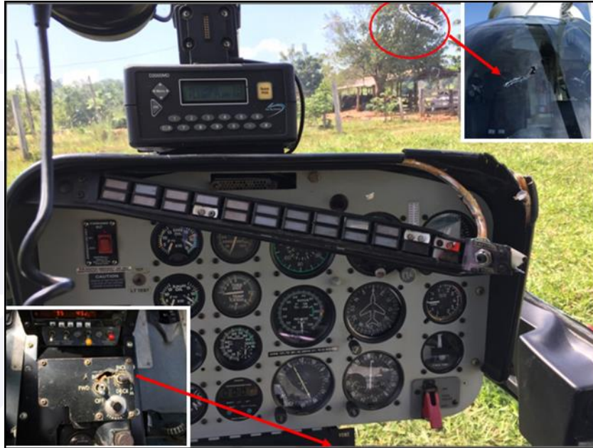
Figure 2 - Panel, windshield and collective with the damages due to the collision against the wire.
