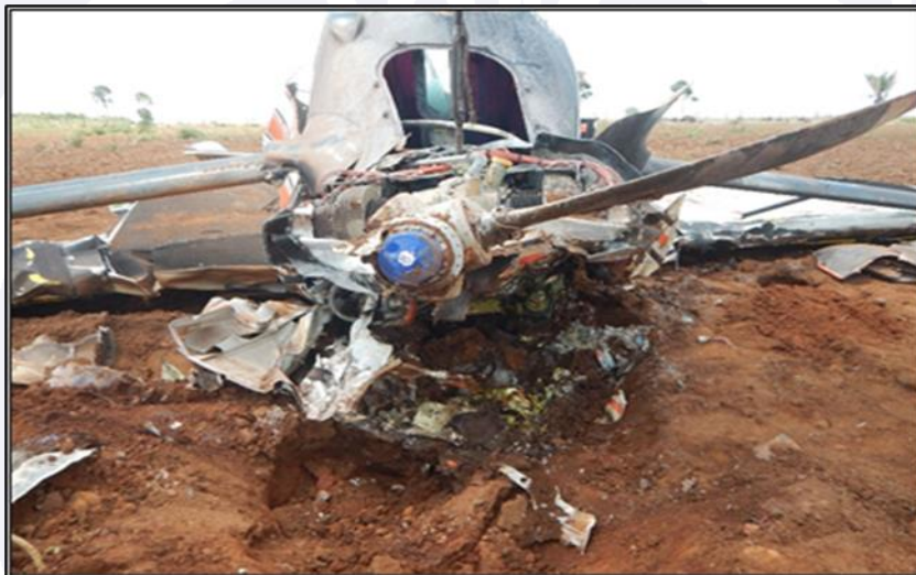
Figure 5 - Propeller with two blades torn from the hub.
