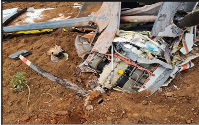
Figure 4 - Engine partially buried, with two propeller blades torn from the fixing hub.
