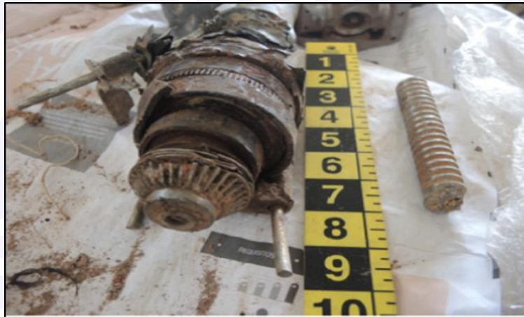
Figure 24 – Horizontal stabilizer electric engine and jackscrew section.
