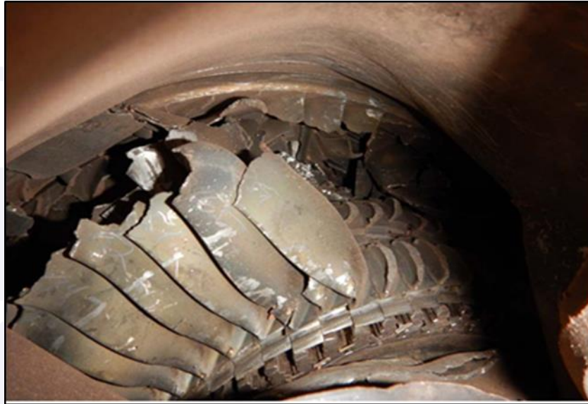
Figure 26 - Damaged blades of the right low-engine turbine.
