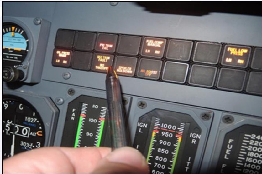
Figure 3 - PRI TRIM FAIL and SEC TRIM FAULT lights on the warning and alarm panel.
