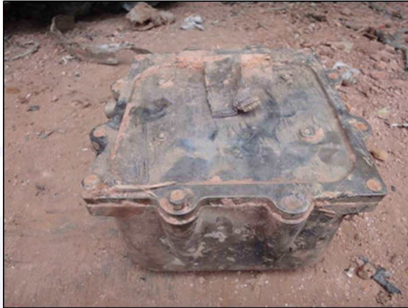
Figure 22 - CSMU at the accident site.
