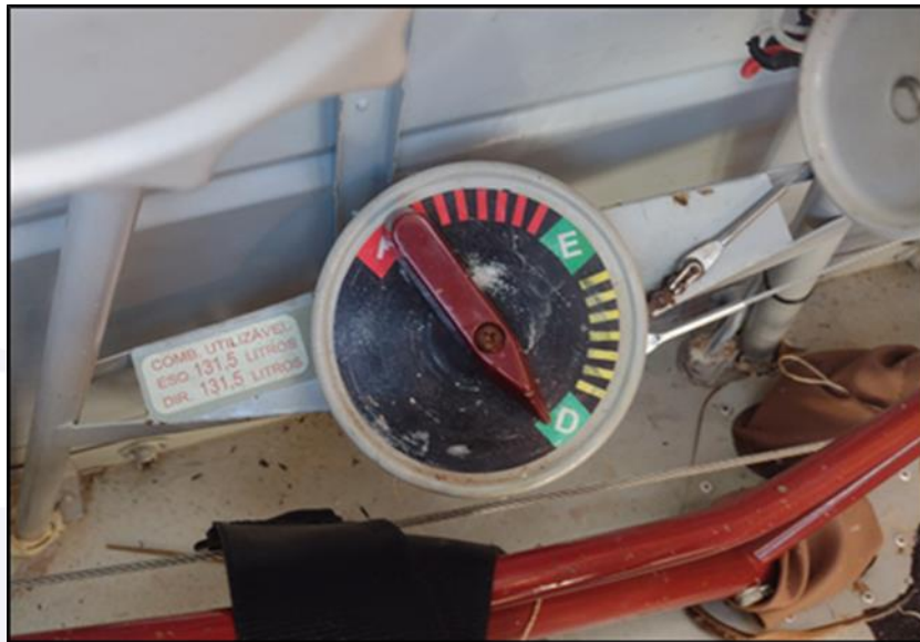
Figure 5 - Fuel tank selector in the "D" position at the accident site.
