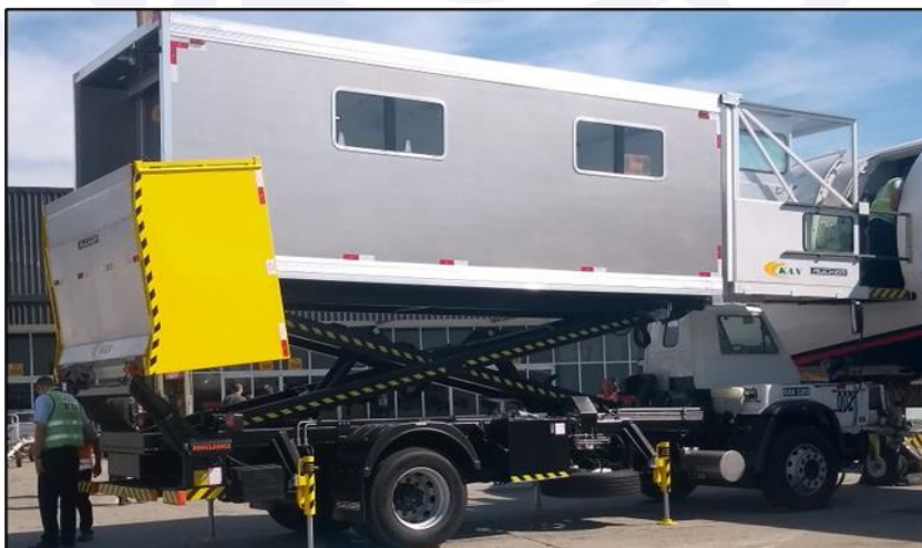
Figure 7 - Image of an Ambulift equipment used for boarding and disembarking passengers, with mobility difficulties, in SBGR.
