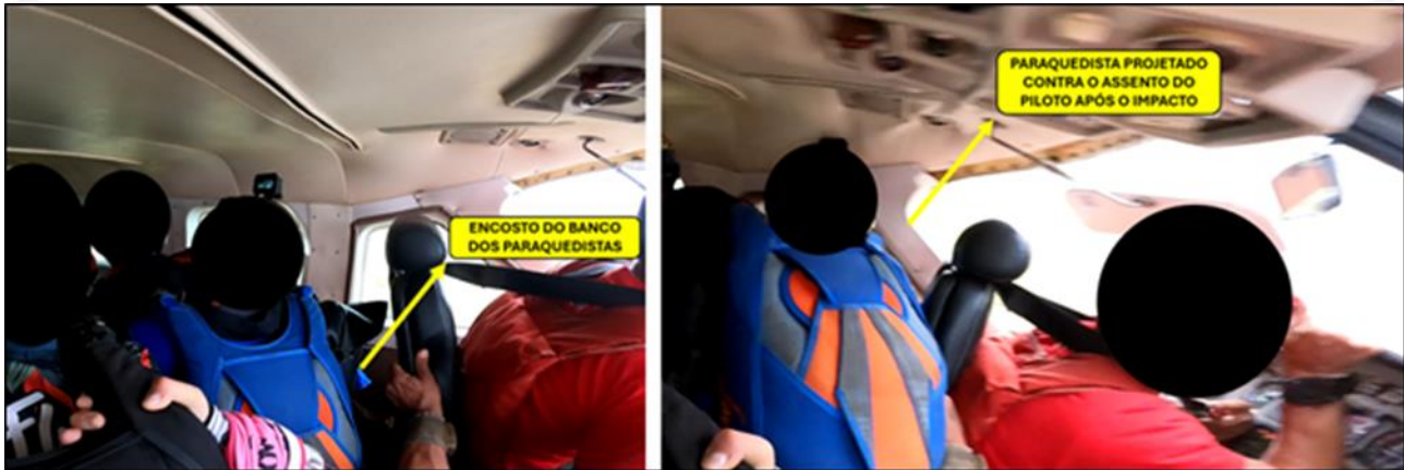
Figure 23 – First parachutist on the left bench of the aircraft (closest to the pilot) with back away from the seat backrest, pre-impact (left) and post-impact (right).
