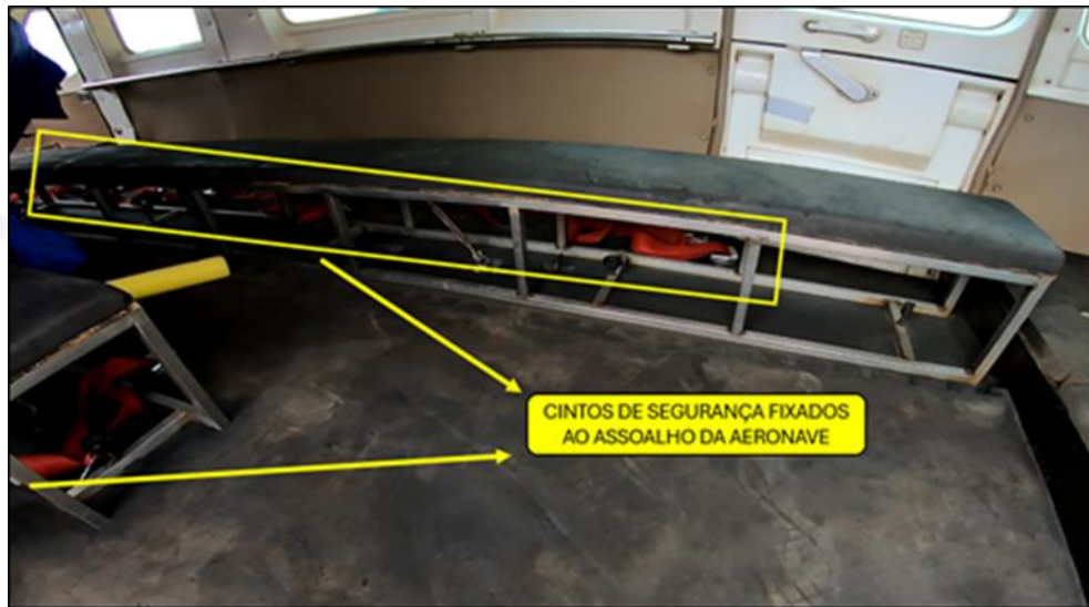
Figure 9 – Highlight showing the positioning of the seat belts attached to the floor on only one side of the benches (outer sides of the cargo cabin).
