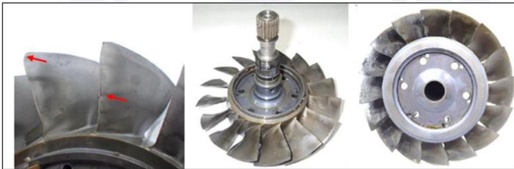
Figure 35 – First stage of the axial compressor; red arrows point to FO-induced damage.
