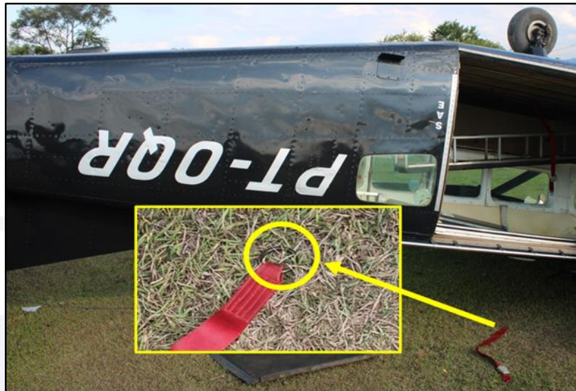
Figure 27 – Seat belt found next to the aircraft, with intact anchor ring.
