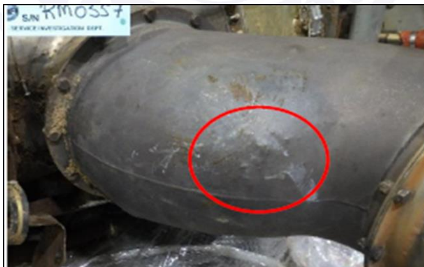
Figure 31 – Damage observed on the aircraft's left exhaust duct.
