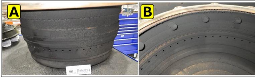
Figure 37 – Internal and external lining of the combustion chamber showing soot deposits and carbon buildup on the walls and cooling ring.
