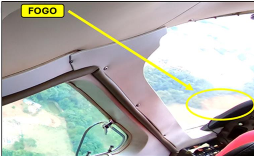
Figure 25 – Flames visible from the left exhaust moments before the emergency landing.
