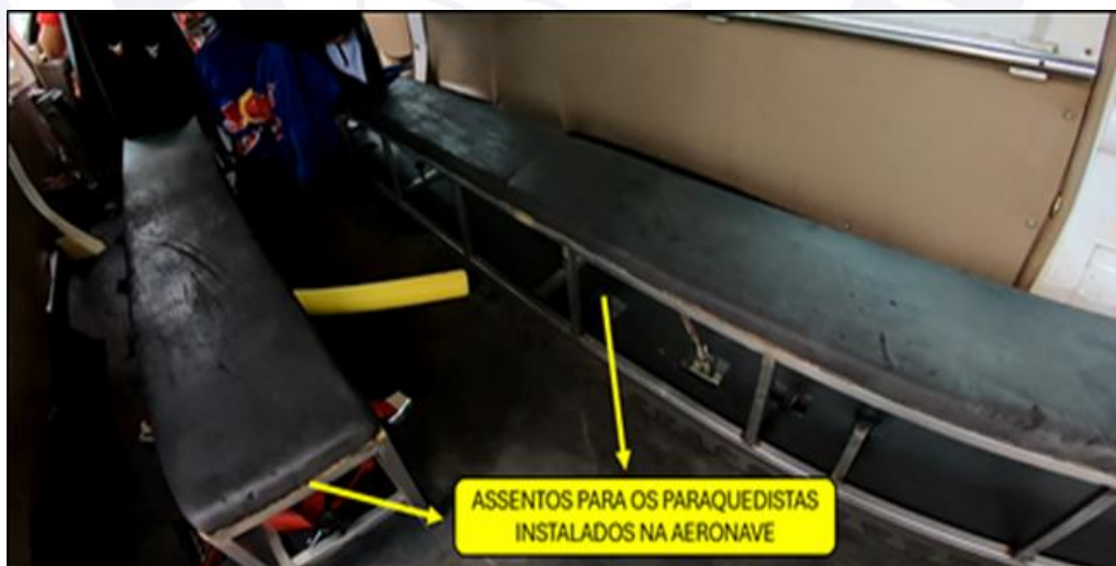
Figure 8 – Internal configuration of the aircraft for the transport and drop of parachutists during the accident flight.
