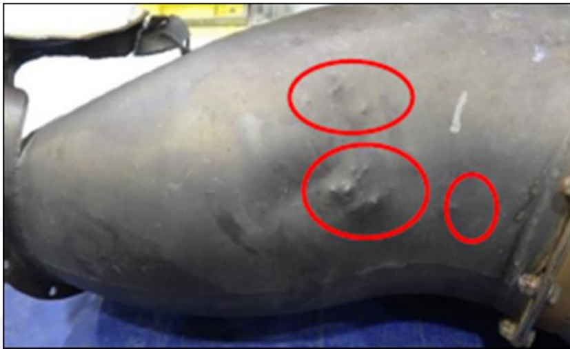
Figure 32 – Damage observed on the aircraft's left exhaust duct.
