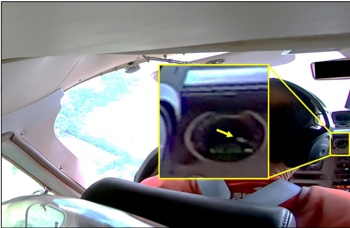
Figure 43 – ITT indication near the instrument's upper limit.
