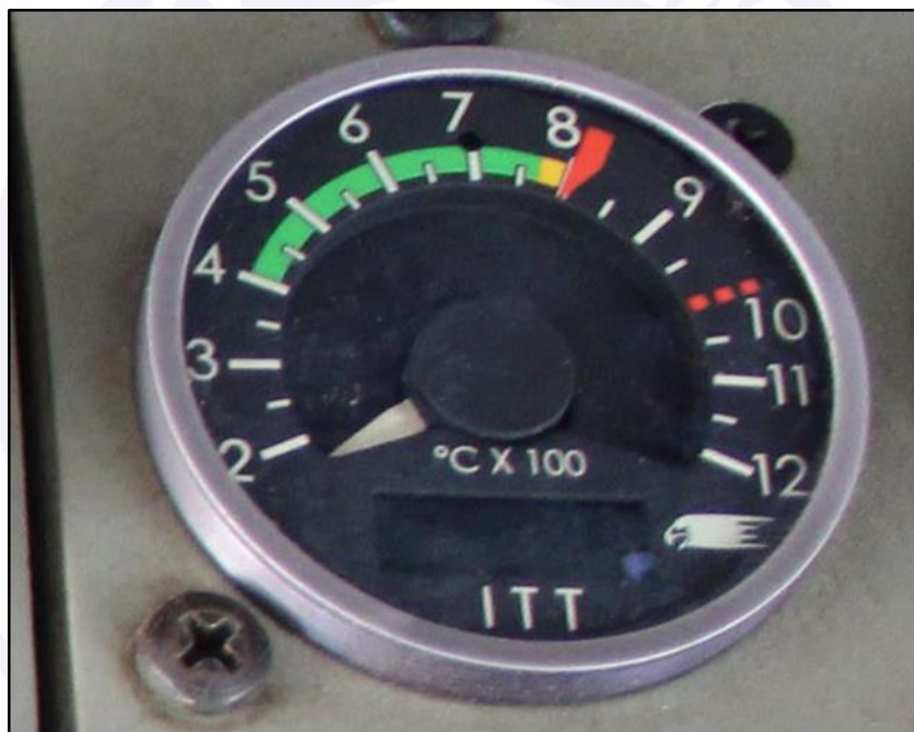
Figure 44 – Photo of the ITT indicator taken after the accident.
