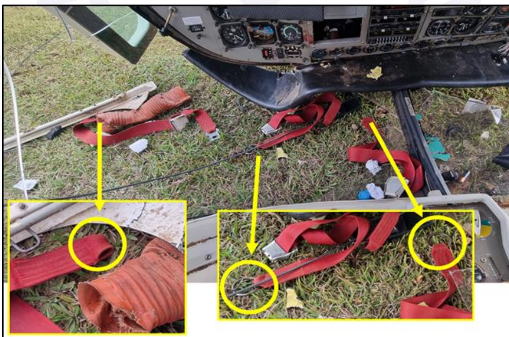
Figure 26 – Seat belts found at the front of the aircraft: missing anchor ring (highlighted on the left) and with intact anchor rings (highlighted on the right).
