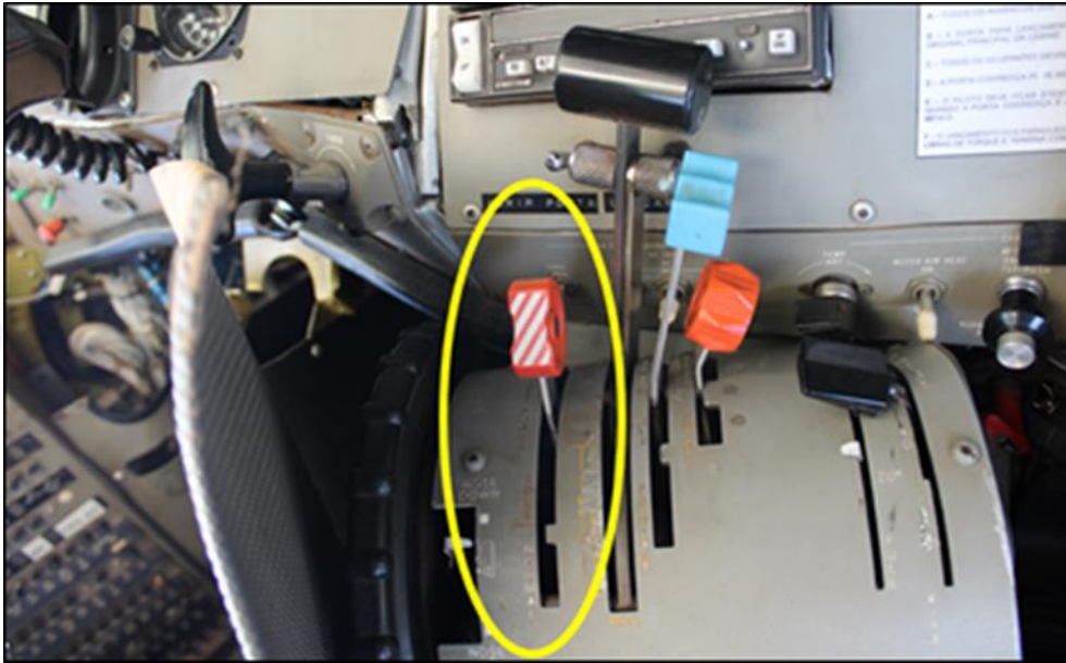
Figure 5 – Throttle quadrant of the PT-OQR after the accident, highlighting the EPL.
