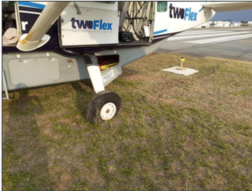
Figure 2 – Left-hand side view of the aircraft. It is possible to observe damage to the wheel-tyre set, and the final position of the aircraft after overrunning the RWY end.
