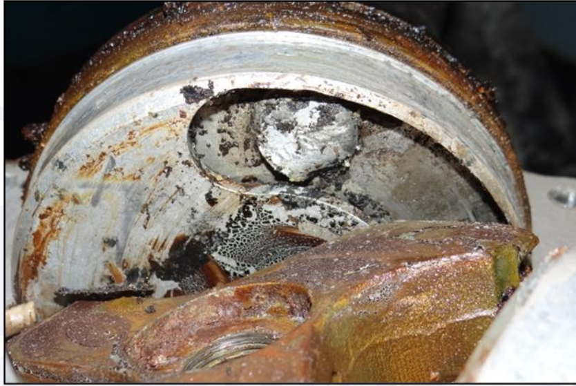
Figure 16 - View of the overload rupture of the blade pitch change pin.
