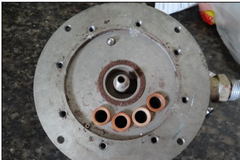
Figure 11 - General view of the fuel selector valve communication holes with the aircraft's fuel tanks.
