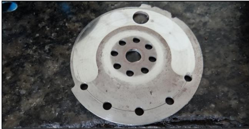
Figure 10 - Face of the fuel selector valve disc with clean area.
