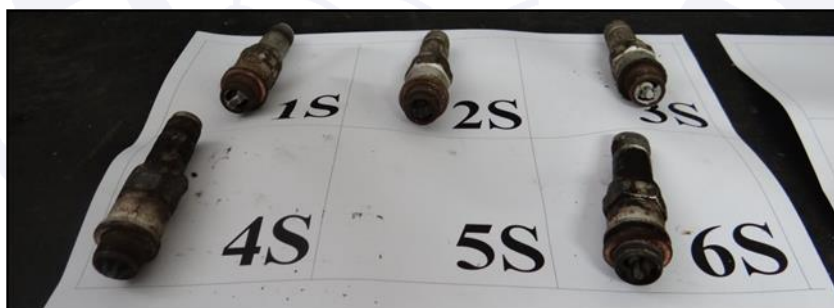
Figure 13 - View of the upper igniters of cylinders 1, 2, 3, 4 and 6.
