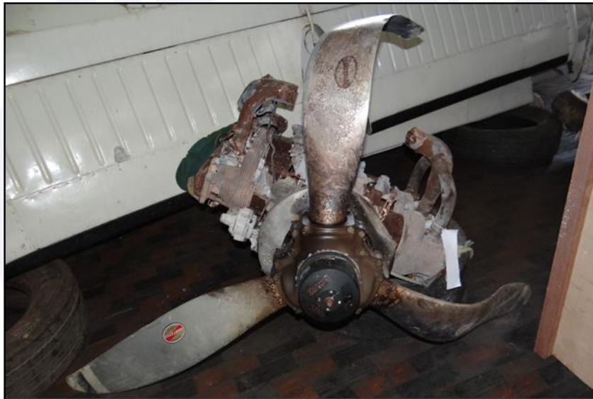
Figure 14 - Front view of the Hartzell HC-C3YR-1RF propeller still mounted on the engine.
