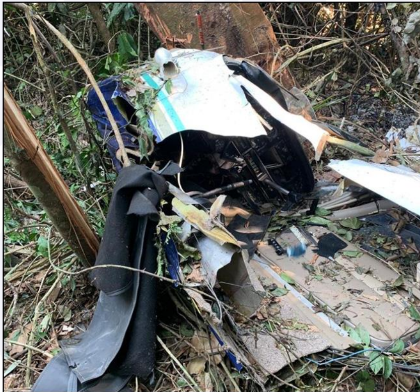
Figure 7 - Cabin front structure with the aircraft panel.
