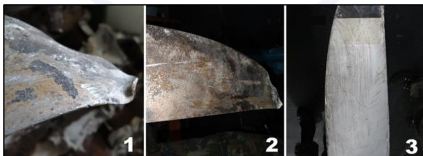
Figure 15 - View of forward-facing bends at the end of two blades and longitudinal scratches at the third.
