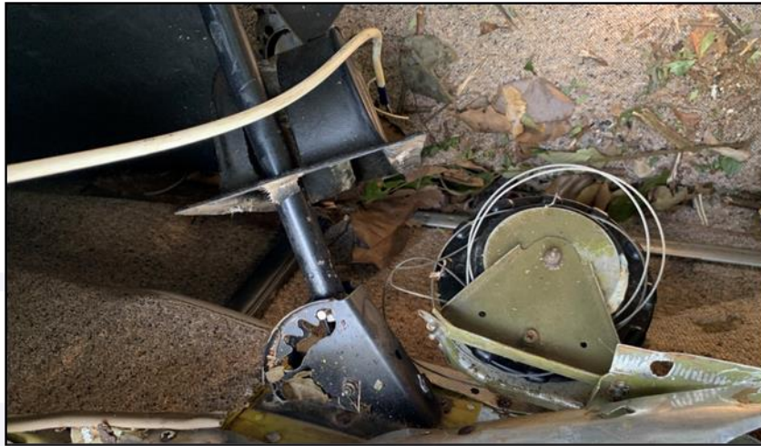
Figure 12 - View of the flap control lever at 40-degree position.
