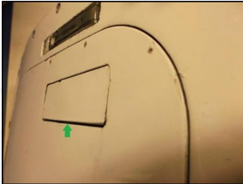
Figure 2 - External view of the small flap partially open, after closing by electric activation.
