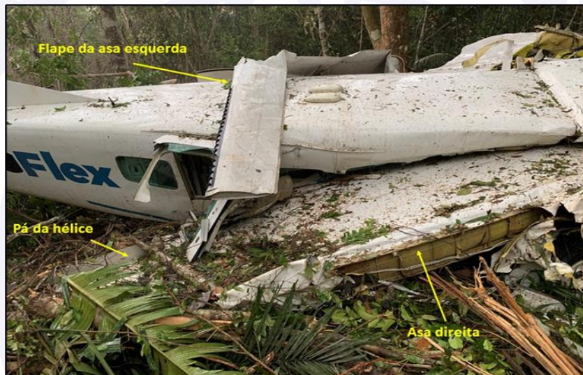
Figure 24 - Close-up view of the right side and top of the aircraft. In the details, the position of the right-wing, the left-wing flap, and a blade of the propeller assembly.
