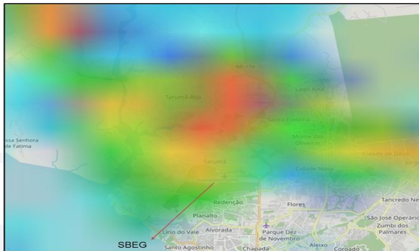
Figure 12 - Close-up image of the meteorological RADAR at 1625 (UTC). The meteorological formation existing in the vicinity of SBEG is observed, with an intensified and more comprehensive red color, indicating strong reflectivity and precipitation.
