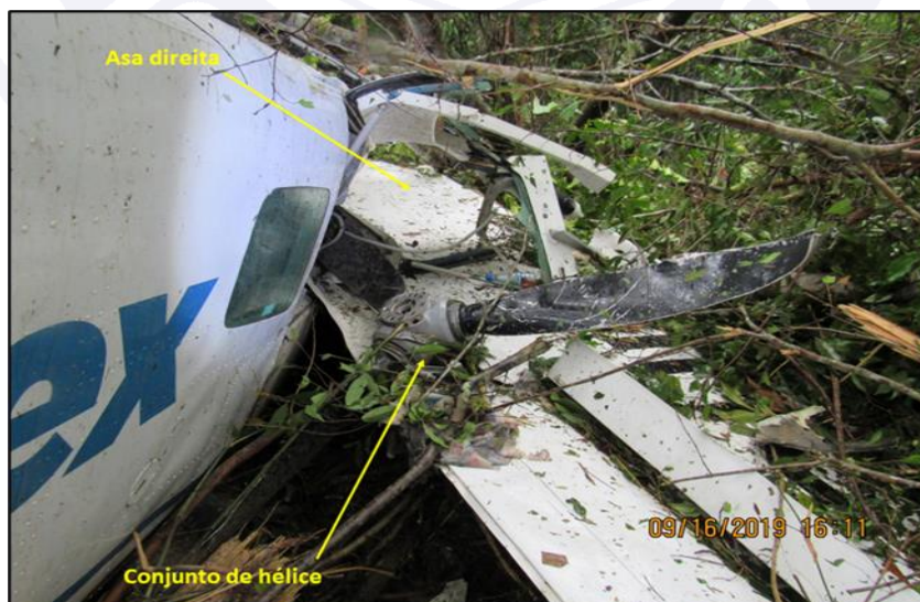
Figure 25 - Close-up view of the right side of the aircraft, near the passengers` door. In the details, the position of the right-wing and the final position of the propeller assembly.
