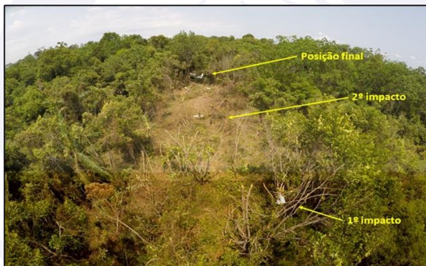
Figure 22 - Aerial view of the accident site. The details show the points of impact and the final position of the aircraft.
