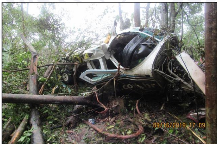
Figure 1 - View of the right front of the aircraft, after the impact and complete stop.
