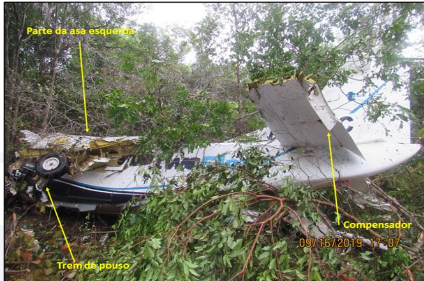
Figure 23 - Close-up view of the aircraft after coming to a complete stop. The yellow arrows indicate the position of the left landing gear, the broken elevator trim, and the part of the left wing that has bent up from the aircraft.
