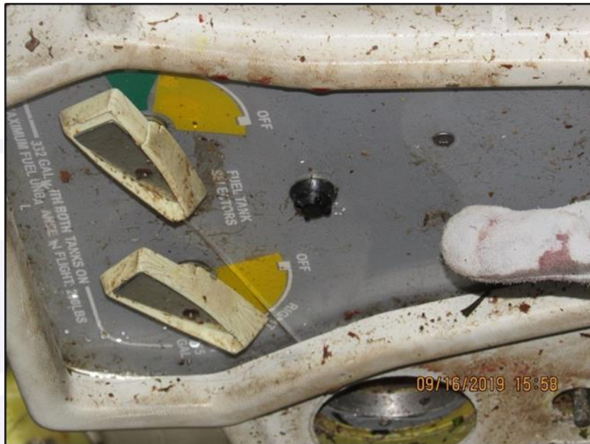
Figure 28 - Close-up view of the fuel selector panel. The selectors were moved by the impact.
