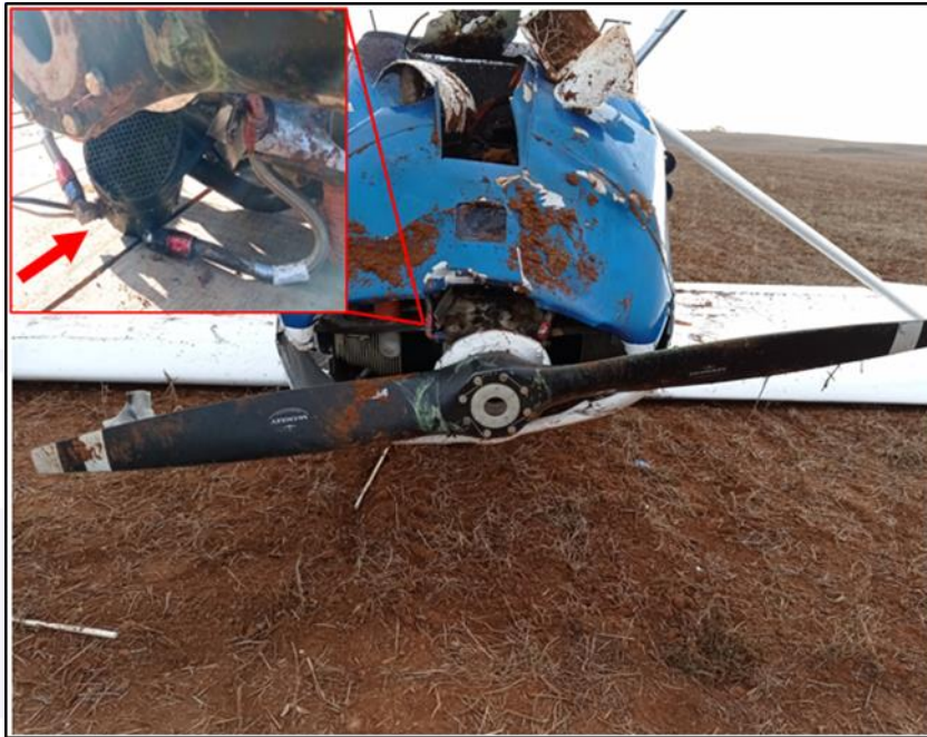
Figure 4 – Frontal view of PT-KUM. In highlight, the item found after the engine cowling was removed.
