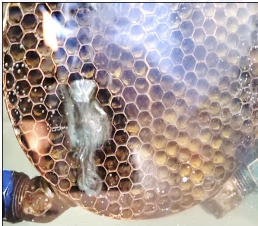
Figure 7 – Detail of the area with leakage.
