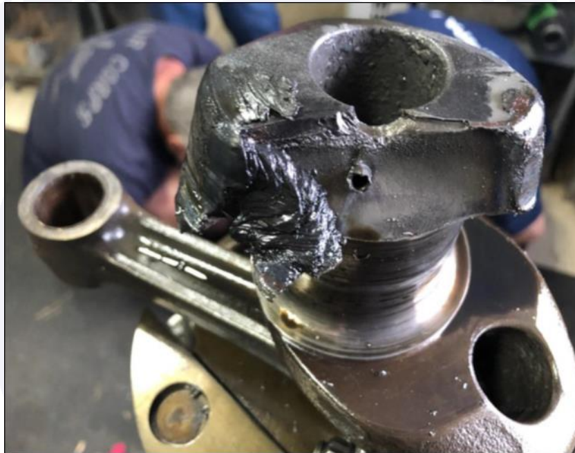
Figure 7 - Fracture in the crankshaft.
