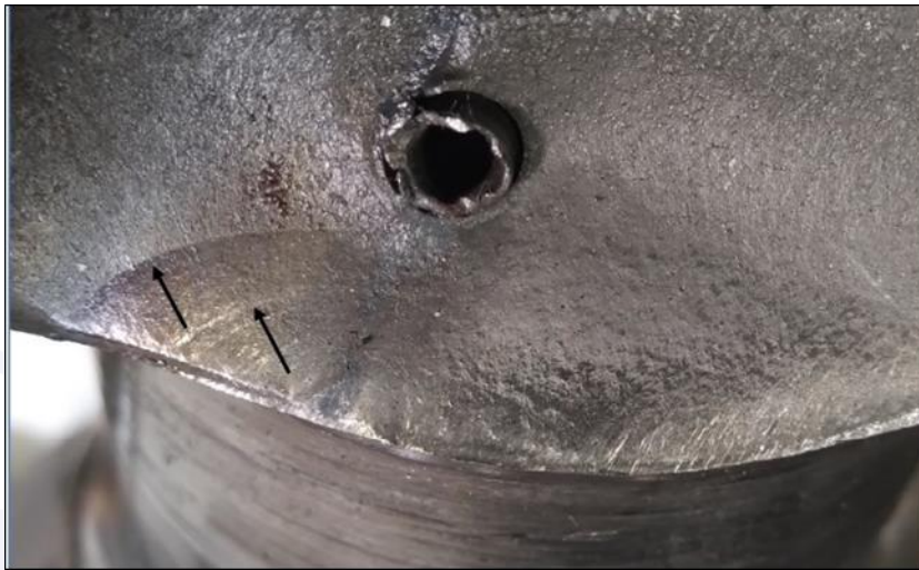
Figure 9 - Examination by means of stereoscopy. In the detail of the fracture surface, one observes beach marks indicative of fatigue (arrows).
