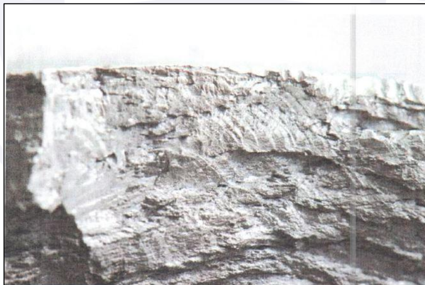
Figure 11 - Propeller-hub fracture surface showing characteristics of fatigue.
