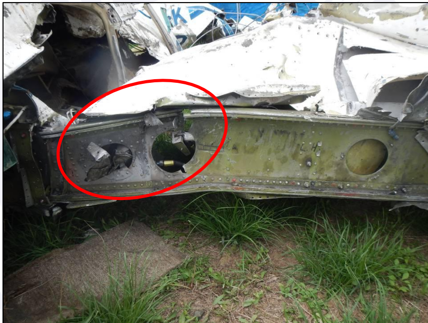
Figure 7 - Aspect of the left wing spar at the point of attachment of the engine nacelle.
