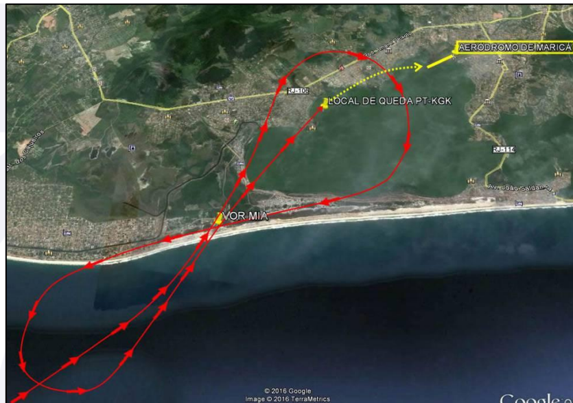
Figure 1 - Illustration of the aircraft trajectory over MIA VOR and Maricá Lagoon (solid red line) and the intended route for landing in Maricá Aerodrome (after the point where the crash occurred).
