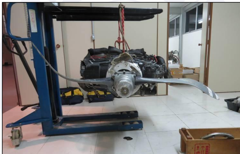
Figure 9 - Number-2 engine bent propeller blades.
