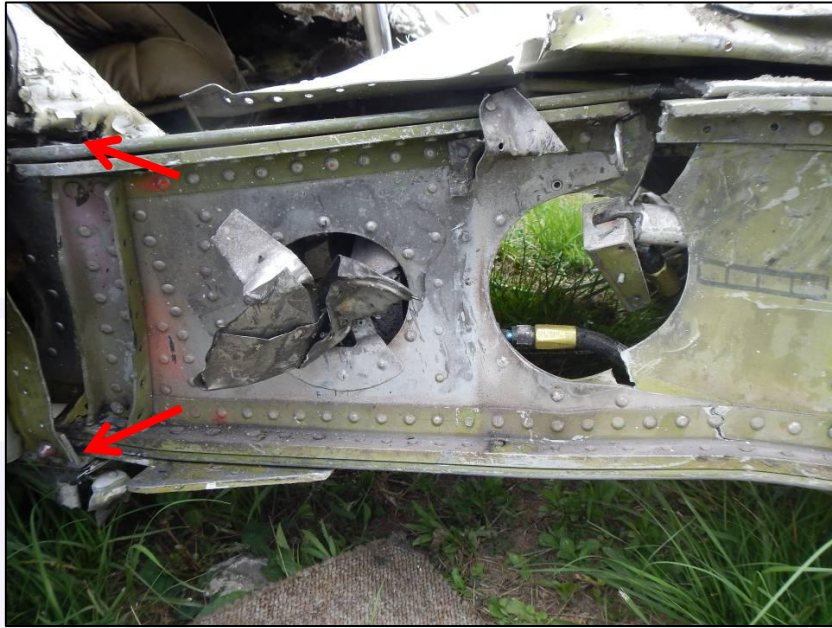
Figure 8 - Aspect of the engine nacelle attachment points.
