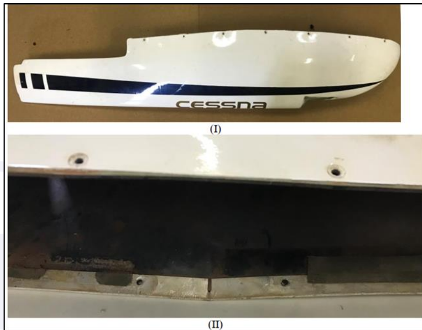
Figure 27 – Right-wing tip that ha equipped the aircraft prior to the accident (I); detail of the holes for fairing attachment (II).
