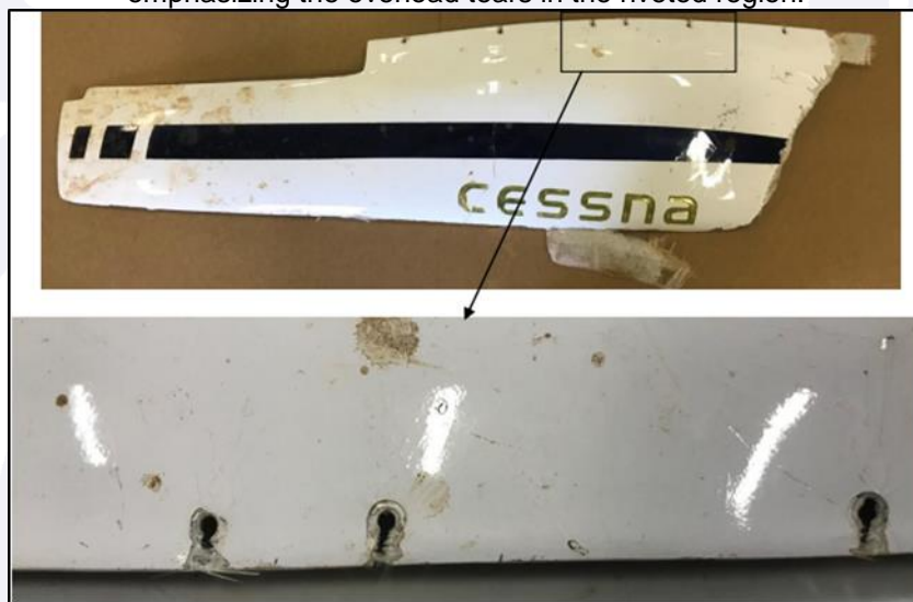
Figure 26 - Details of the right-wing tip fairing, emphasizing the overload tears in the riveted region.
