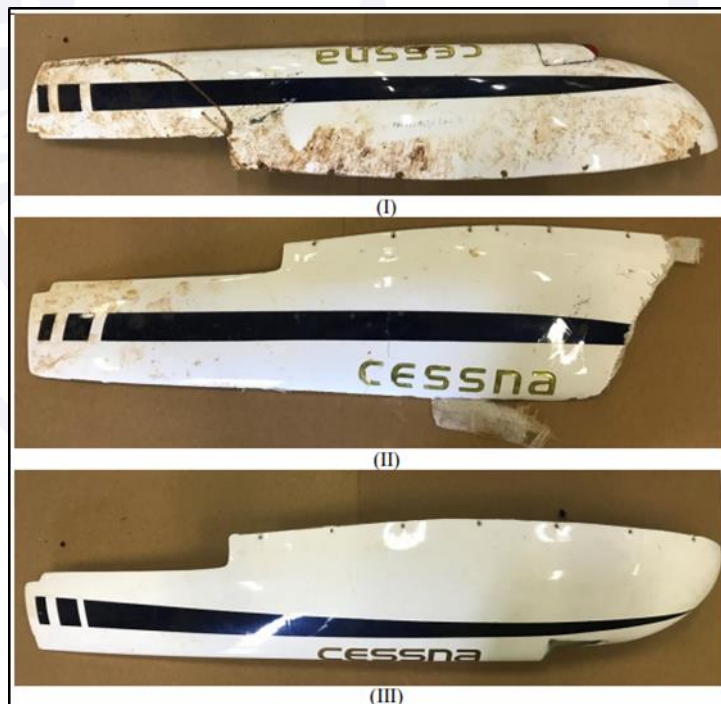
Figure 24 - Fairing of the left-wing tip (I); fractured fairing of the right-wing tip (II); and original fairing that had equipped the PT-KCK prior to the accident (III).
