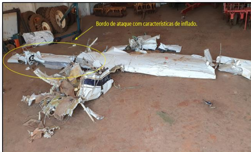
Figure 21 - View of the aircraft, reassembled after the initial action, with details on the leading edge of the right wing, which showed characteristics of inflation.
