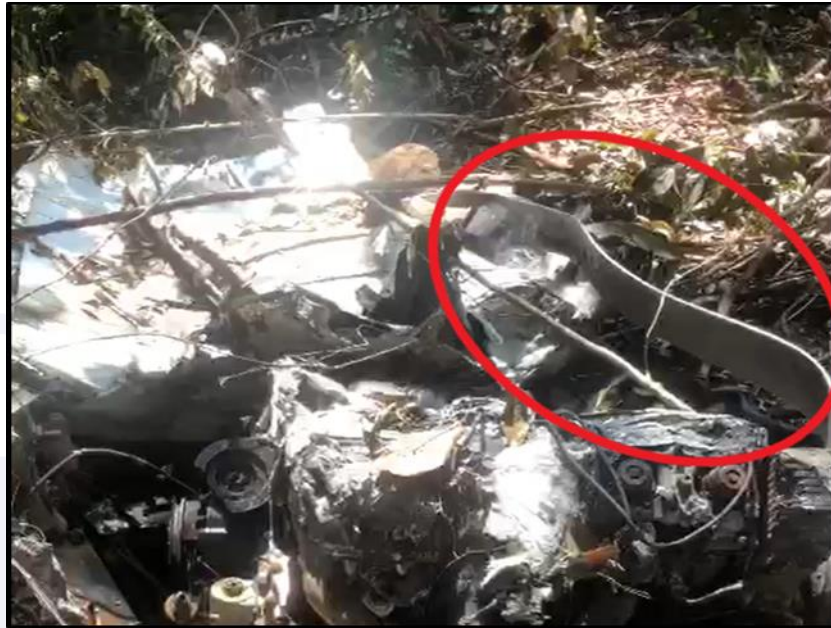
Figure 7 – Aircraft powerplant and one of the propeller blades in highlight.
