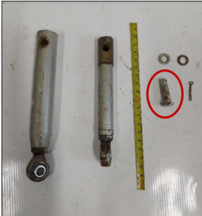
Figure 5 - Photo of the disassembled rod. In the red detail, the pin that was analyzed.
