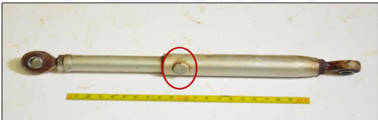
Figure 4 - Photo of the rod removed from the aircraft. In the red detail, the safety pin that did not break and did not allow the emergency procedure to be carried out.
