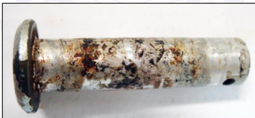
Figure 6 - Photo of the pin without any sign of deformation.
