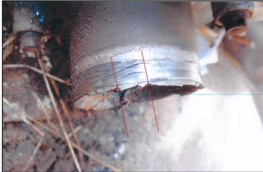
Figure 7 - Crankshaft rupture cracks.
