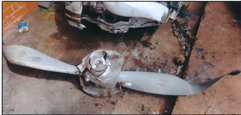
Figure 8 – Bending on the propeller blades.
