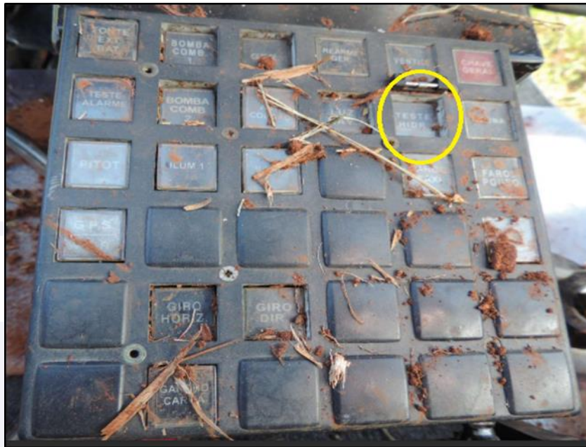
Figure 7 - View of the depressed hydraulic-test (TESTE HIDR) pushbutton.
