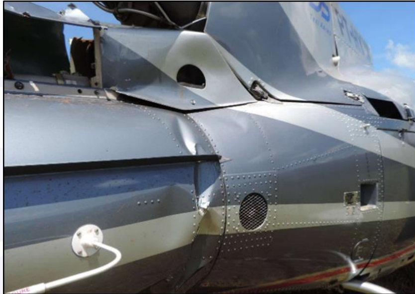
Figure 2 - Damage to the PT-HYW tail boom.
