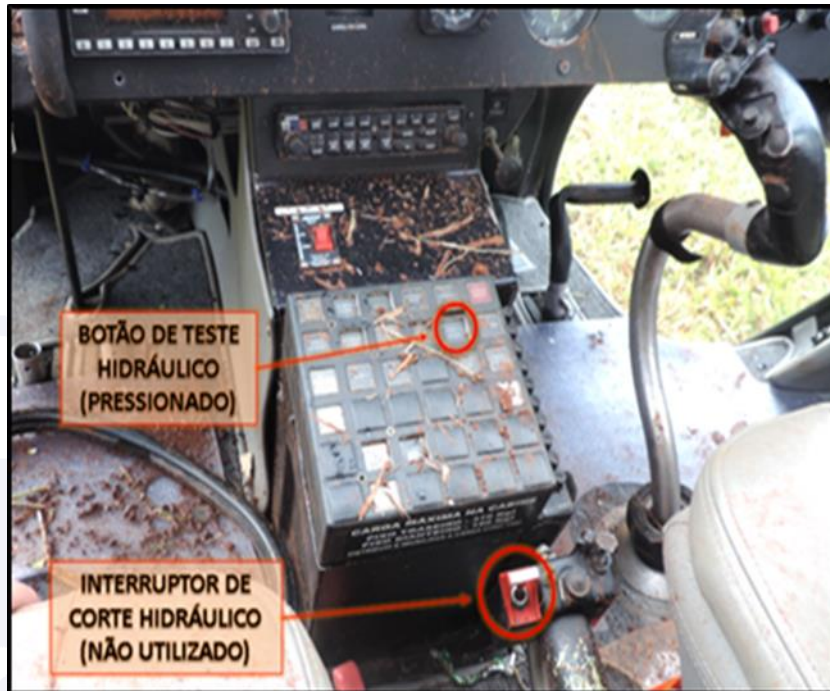
Figure 24 - Final position of the center-console button-panel, and the PT-HYW hydraulic cut-off switch.
