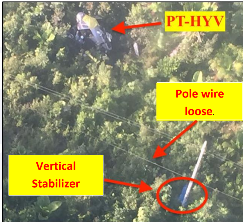
Figure 7 - Aerial view of the aircraft at the accident site, with emphasis on the pole and the vertical stabilizer.
