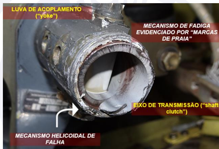
Figure 3 - Detail of the crack formation in the helical direction, in the transmission shaft.
