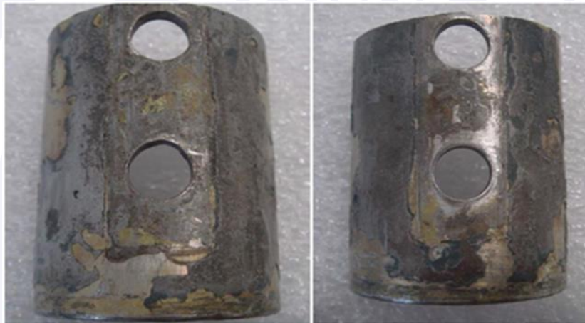
Figure 9 - Aspect of the regions of the axis where the external support blocks are placed. It is noted that the ink was not removed from the settling region of the blocks.
