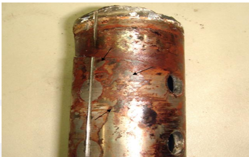
Figure 5 - Fretting marks on the fractured power transmission shaft, with no trace of product applied for protection.
