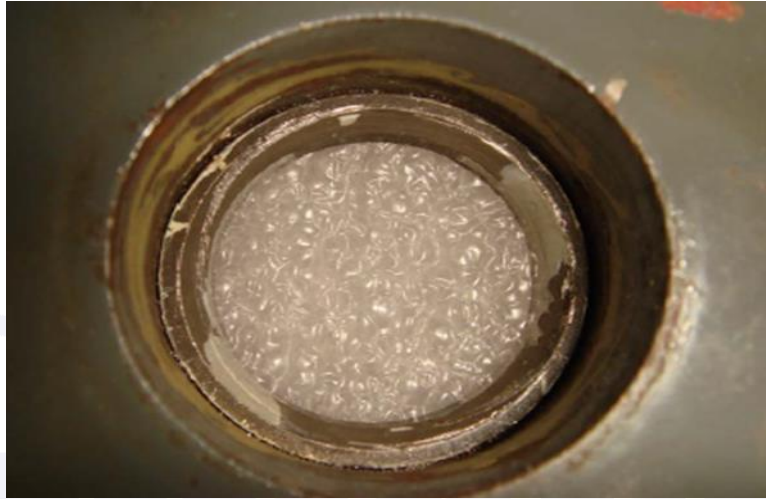
Figure 8 - Rear view of the set: yoke - transmission shaft. It is noted that there was no sealing with primer.
