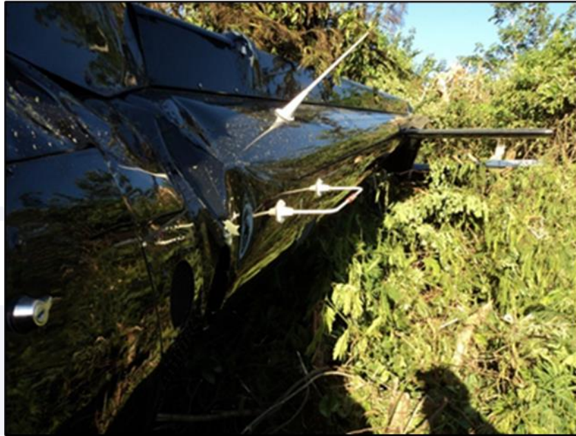
Figure 2 - View of the wrinkled tail cone.
