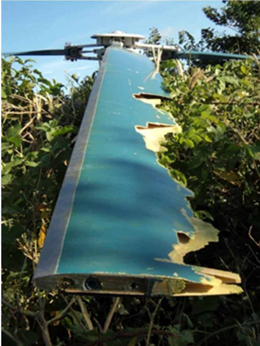
Figure 5 - Main rotor blade broken at the trailing edge.
