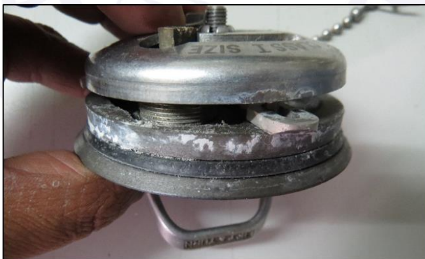
Figure 2 - Condition of the cap sealing-gasket.
