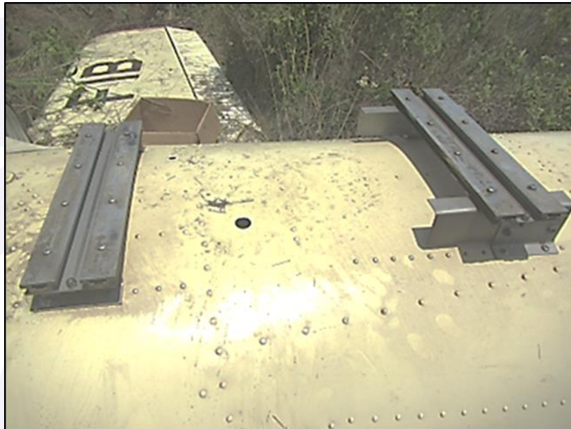
Figure 2 - Metallic structure fixed to the fuselage's underside.
