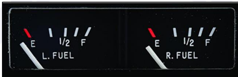
Figure 7 – Close-up view of the fuel indicators. Source: adapted from the plane's Owner's Manual.
