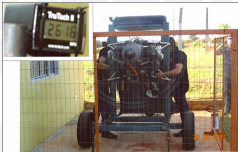
Figure 12 - Engine running at 2,616 RPM during the functional test.
