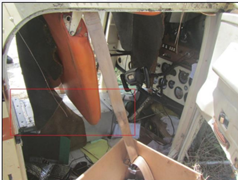
Figure 3 - Metal box that was fixed to the existing structure on the fuselage soffit.
