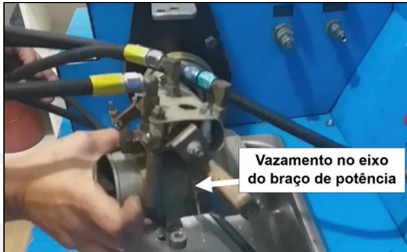
Figure 7 - Leak in the fuel controller power-arm shaft.
