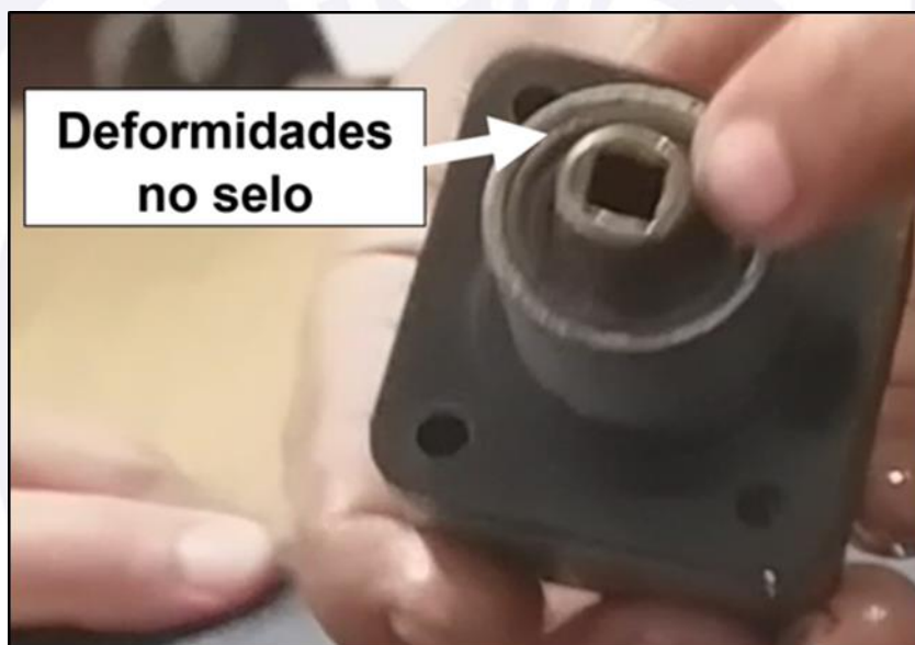
Figure 6 - Retaining seal showing deformities.
