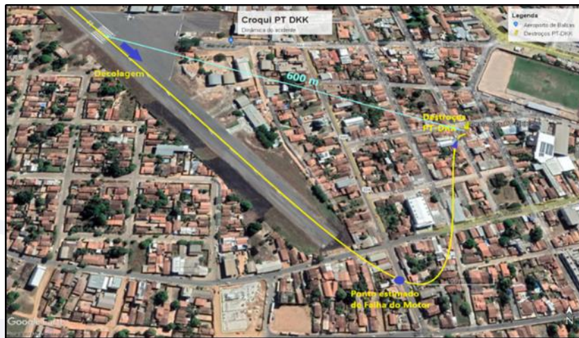
Figure 2 - Croquis showing the distance between threshold 33 and the wreckage. Source: adapted from Google Earth.
