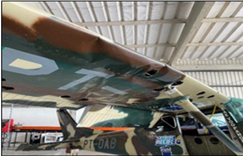
Figure 2 - Damage to the right-hand wing.
