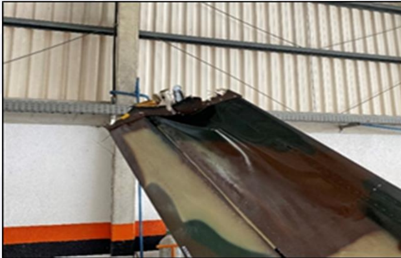
Figure 3 - Damage to the vertical stabilizer.
