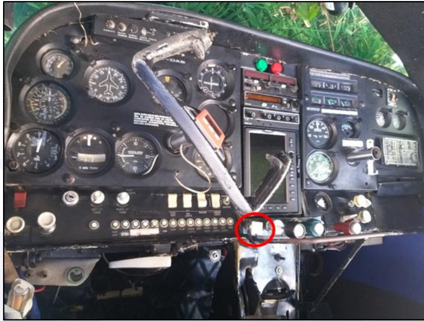
Figure 6 - Detail of the Carburettor Heat lever in the off position.
