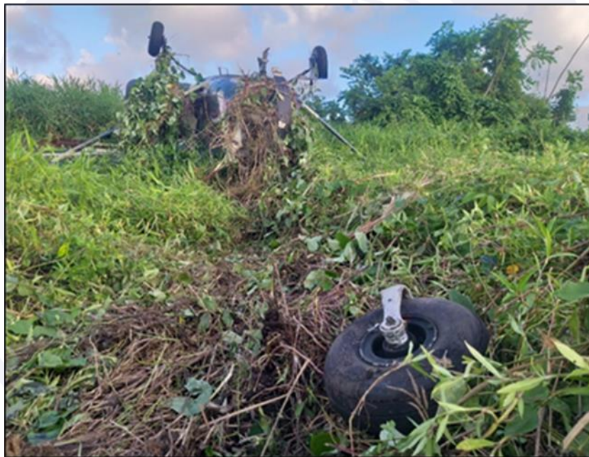
Figure 5 - Auxiliary landing gear separated from the aircraft.
