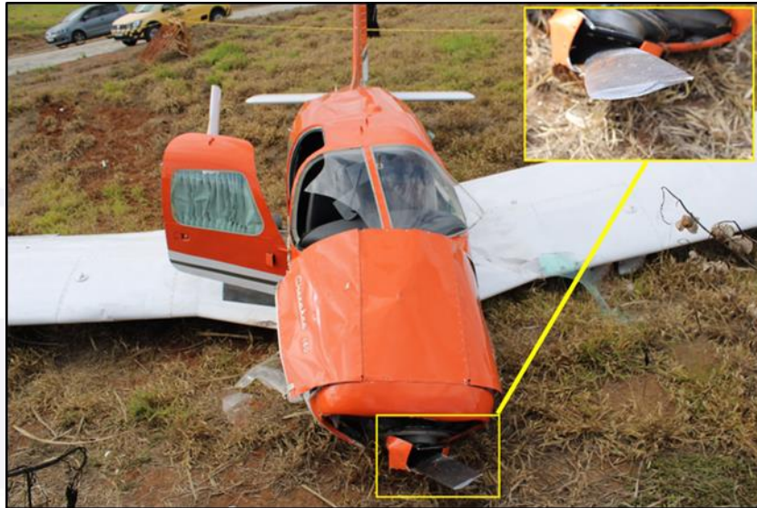
Figure 2 - Close-up image of the damage sustained by the aircraft, and detail of the fractured propeller.
