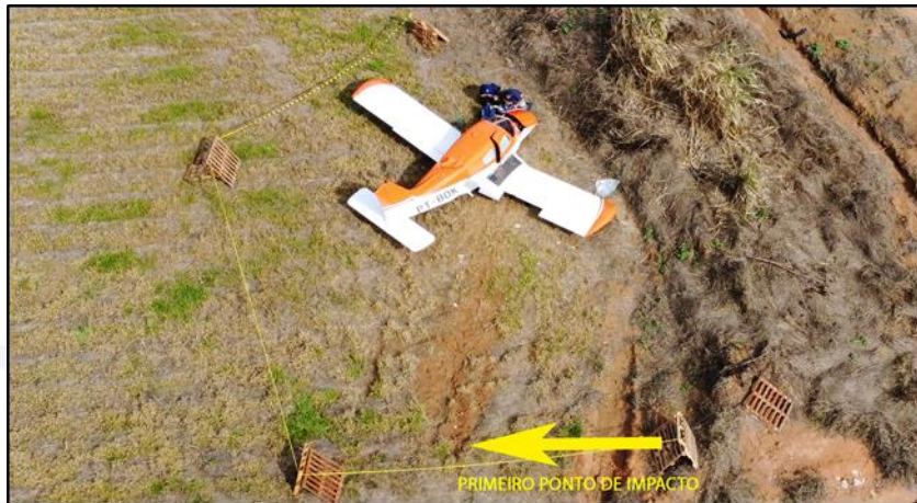
Figure 12 - Marks of the first impact, and final position of the aircraft.
