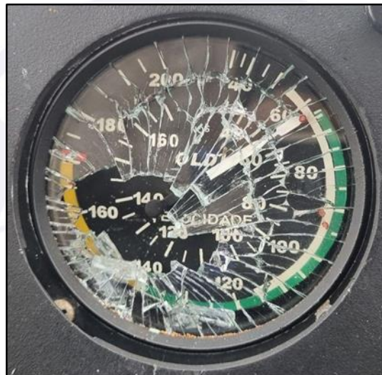
Figure 13 - Indication of the speedometer found in the wreckage of the aircraft.
