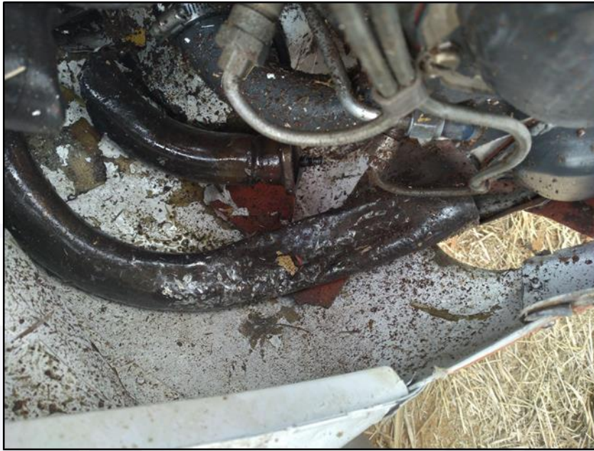
Figure 15 - Part of the exhaust pipes with signs of impact.
