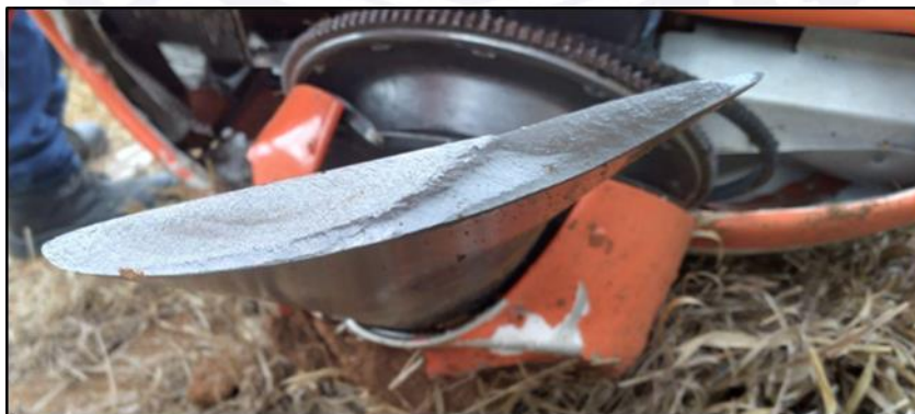
Figure 14 - Fracture in one of the blades.
