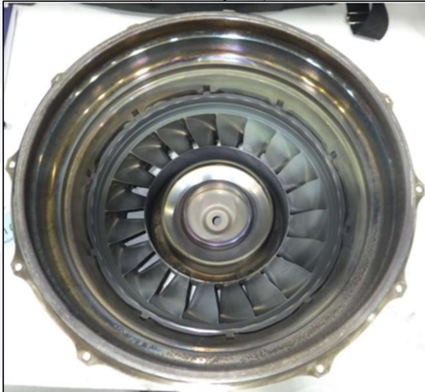
Figure 8 – turbine with discoloration compatible with exposure to high temperatures.
