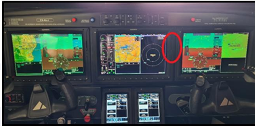
Figure 3 - Panel of the PS-RJJ airplane. Highlighted in red, the position of the SD card slots beside the MFD.
