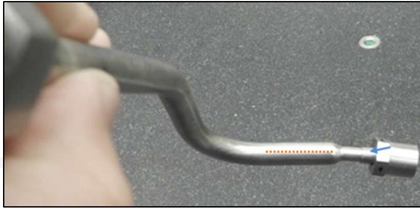
Figure 17 – Deformation at the end of the fuel line closest to the connection with the FCU.
