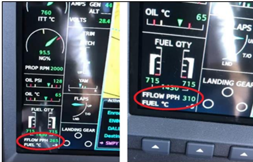
Figure 19 – Images obtained by the pilot after the aircraft levelled off, showing fuel-flow indications at two distinct moments highlighted in red ovals.
