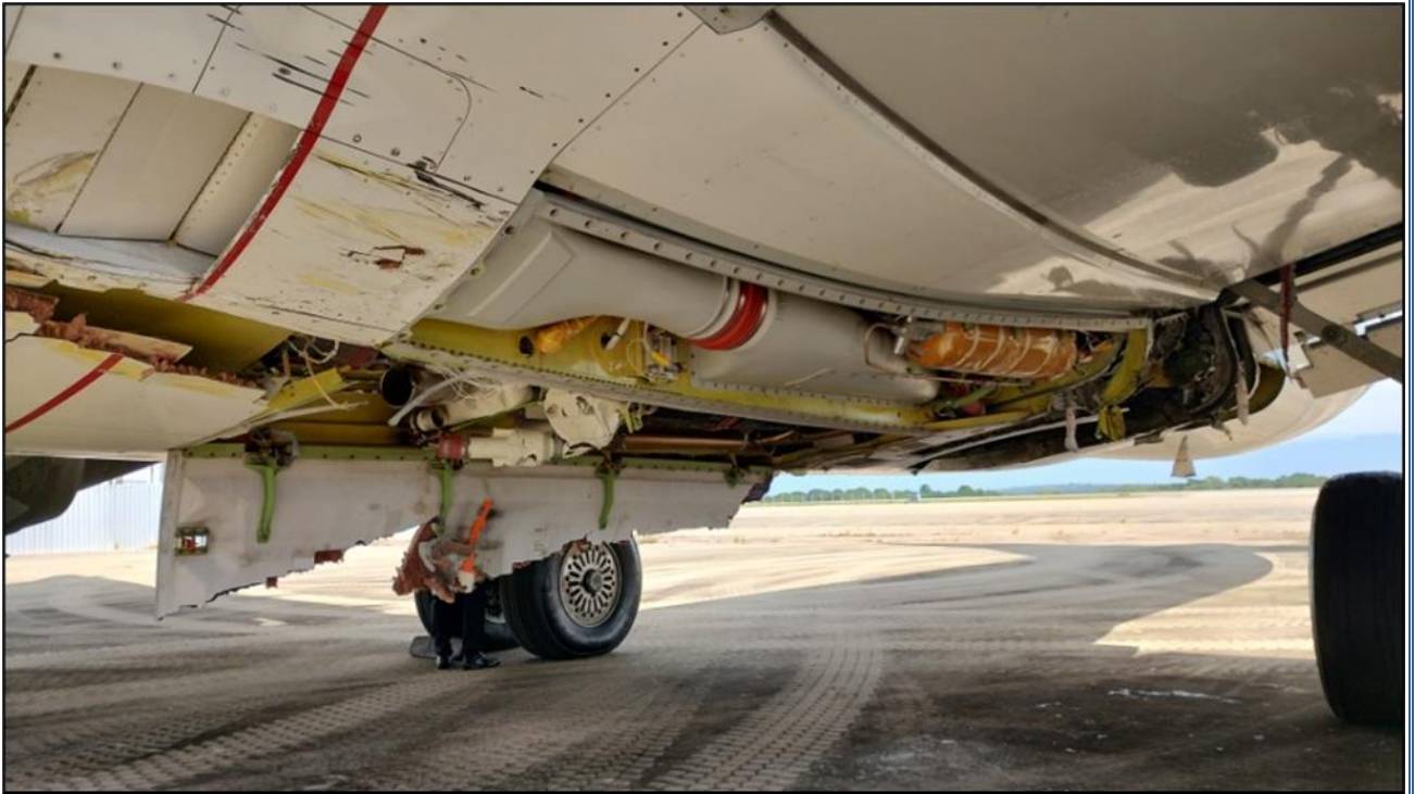
Figure 5 - Damage to the aircraft's lower fuselage fairings.
