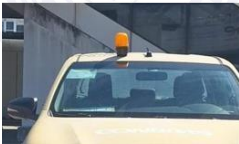
Figure 13 - Lighting pattern used by the vehicle involved in the aeronautical occurrence, featuring rotating and flashing beacons (lightbar) installed on the vehicle roof.
