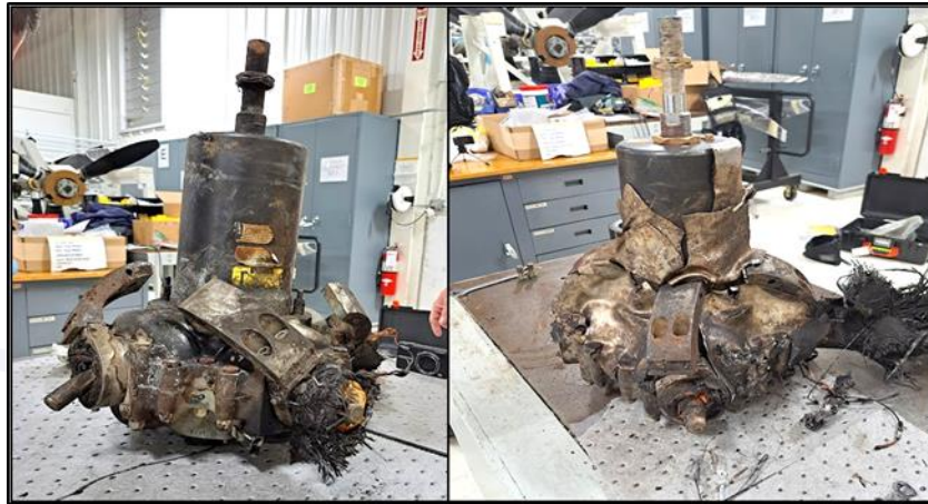
Figure 16 - NR511 (left) and NR505 (right) propeller hubs shown at the beginning of the analyses.
