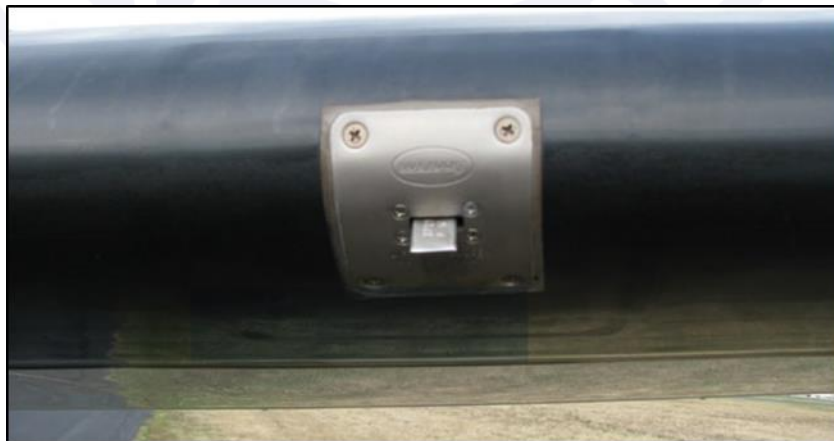
Figure 9 - Stall warning system sensor transducer. Source: aircraft training material - TRU Simulation Training.
