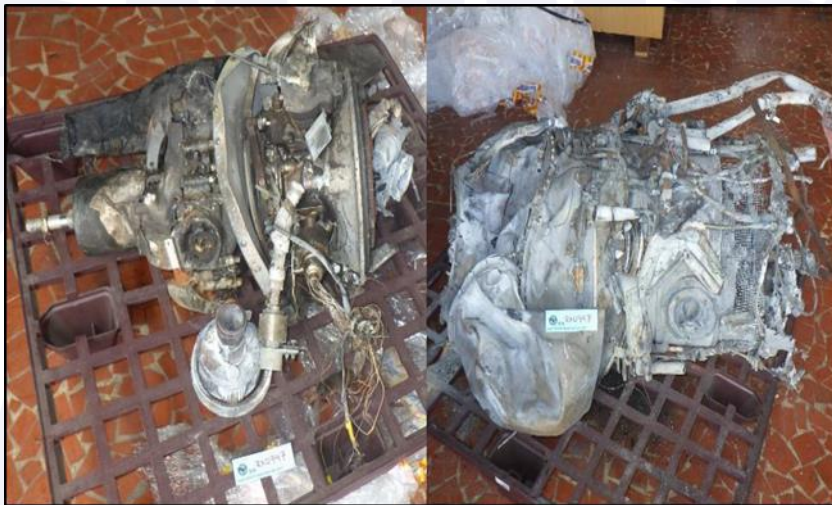
Figure 15 - Right-hand engine (SN RX0947) damaged by impact and fire, separated into two parts at the reduction gearbox.
