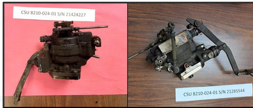
Figure 19 -SN 21424227 and SN 21285544 propeller governors (CSU), during visual inspection.
