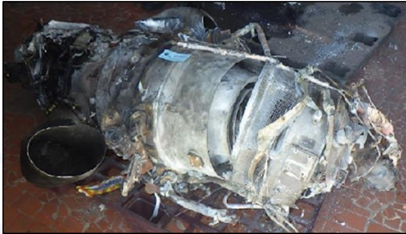
Figure 14 - Left-hand engine (SN RX0972) damaged by impact and fire, showing fracture and partial separation of the air intake.
