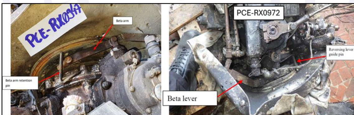
Figure 32 - Positioning of the guide pins in relation to the beta arms on both engines of the PS-CSM airplane.
