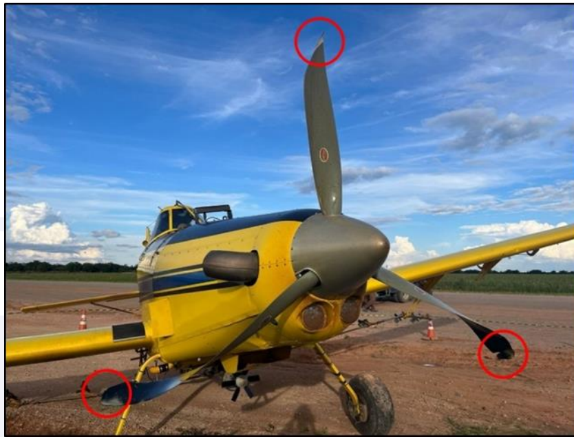
Figure 4 - Damage to the propeller blades.
