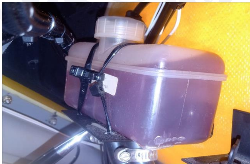
Figure 7 - Reservoir with a full supply of brake fluid.
