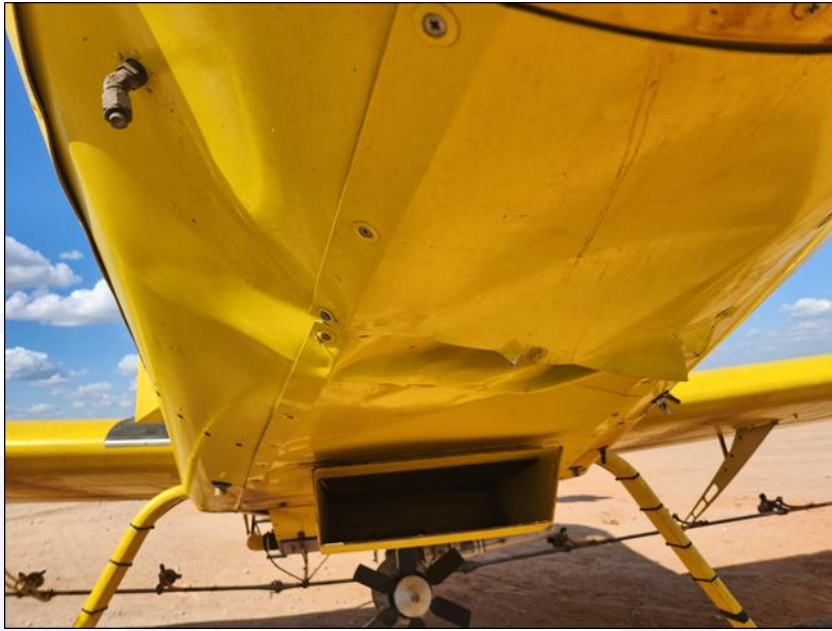
Figure 2 - Damage to the fuselage.
