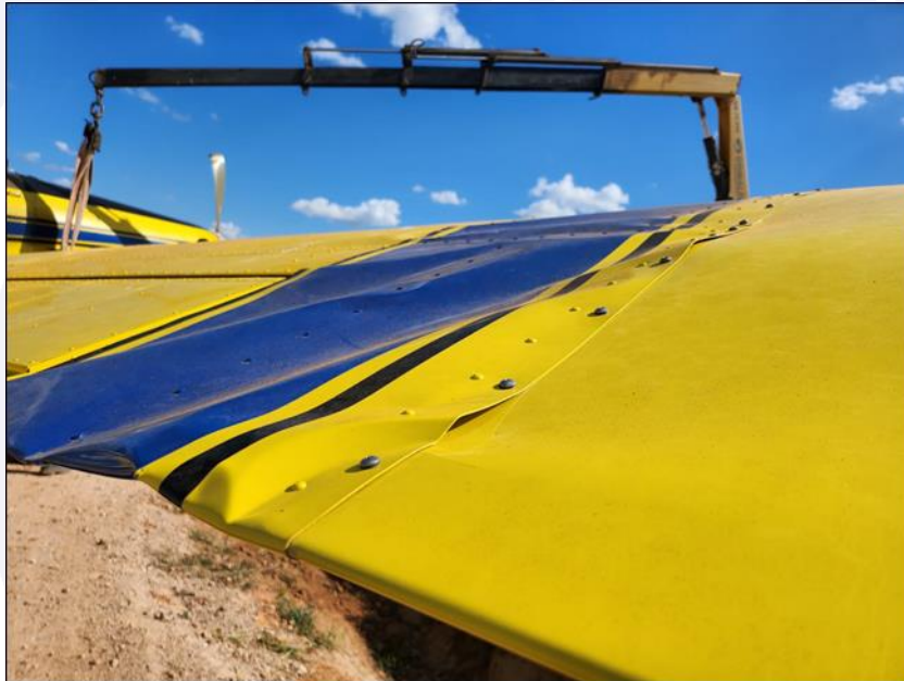
Figure 3 - Damage to the right-hand wing.
