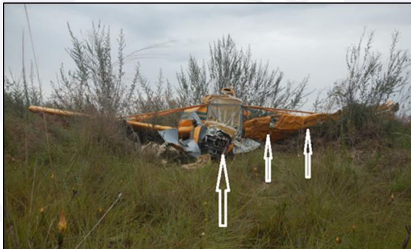
Figure 3 – Front view of the aircraft, with indication of the most severe damaged areas.
