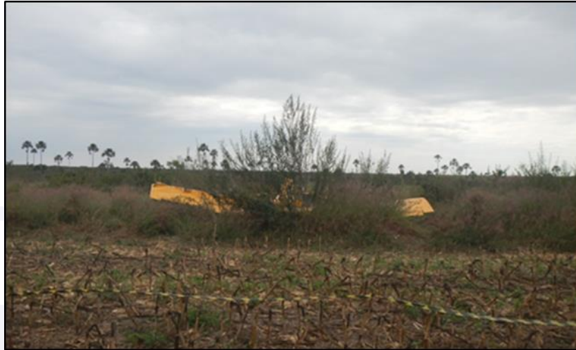
Figure 4 – Rear view of the aircraft, showing absence of signs of horizontal displacement of the wreckage on the ground.
