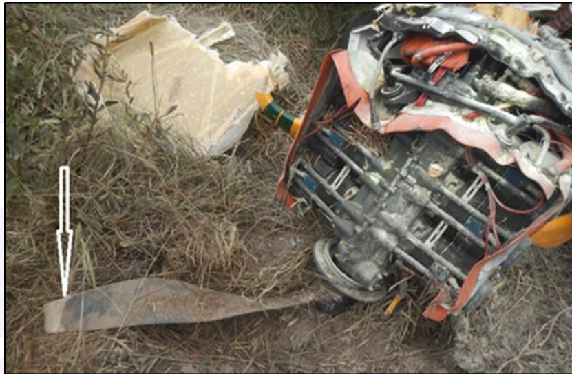
Figure 5 - View of one of the propeller blades, indicating the twisting and folding of the end of the blade forward.
