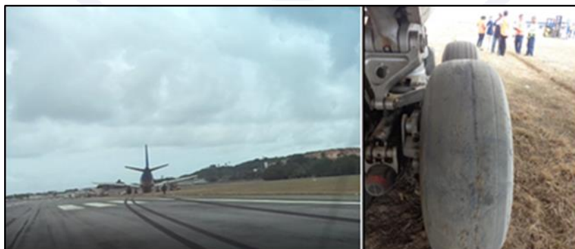
Figure 16 - Marks of the left main landing gear. On the detail, the wear observed on the tires of this landing gear.
