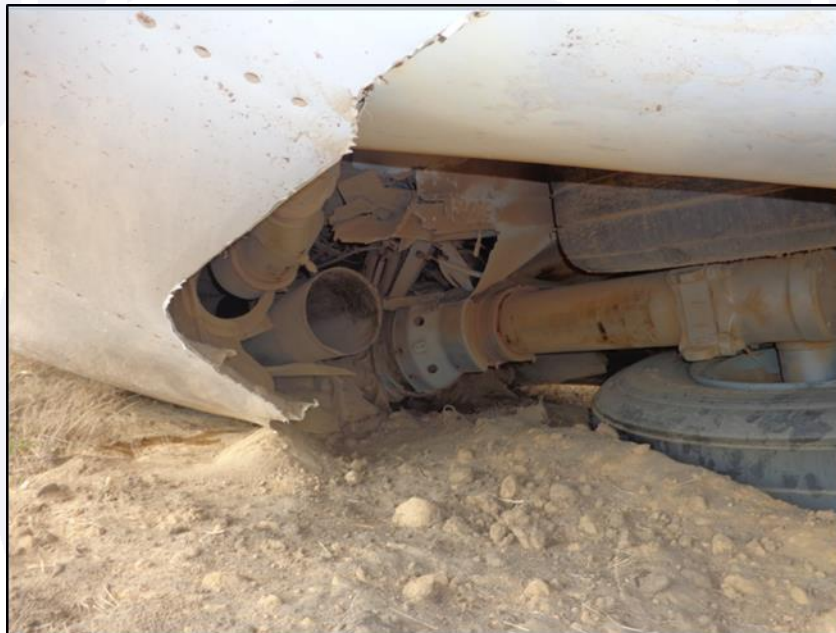
Figure 2 - Detail of damage to the nose landing gear.
