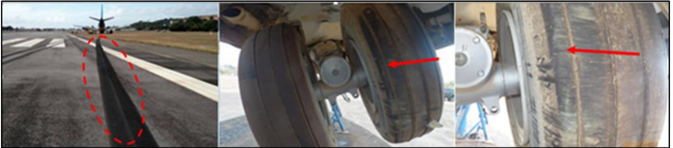
Figure 17 - Nose landing gear marks and tire wear indicating skidding.
