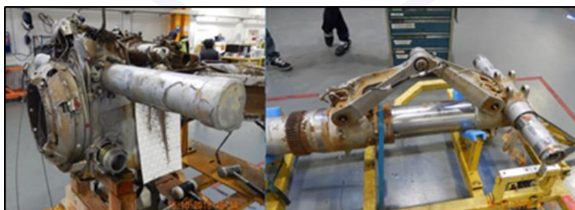
Figure 18 - Landing gear undergoing disassembly for Safran exams.
