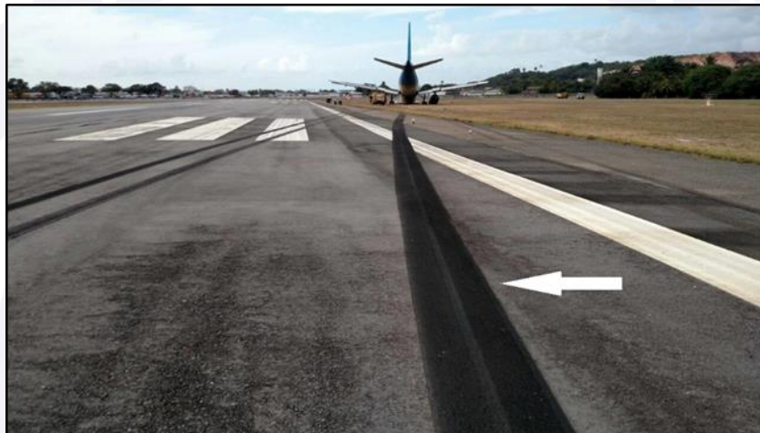
Figure 15 - Overlapping nose landing gear tire markings (white arrow).
