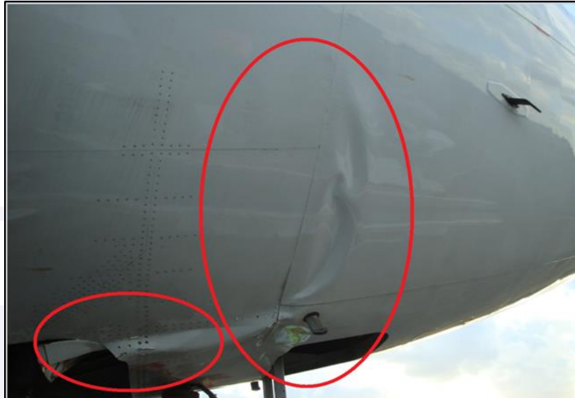
Figure 3 - Details of fuselage damage.
