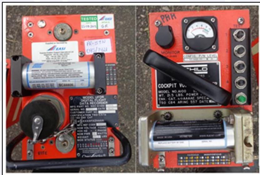
Figure 14 - FDR and CVR after the aircraft removal.
