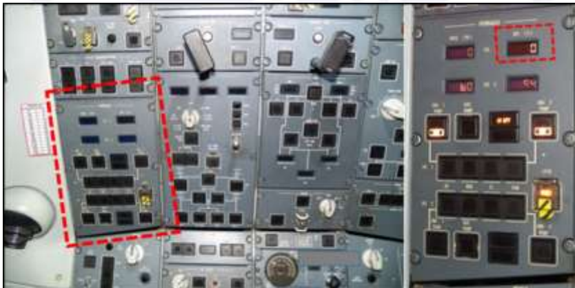
Figure 12 - Hydraulic panel detail and amount of fluid in the system 1.
