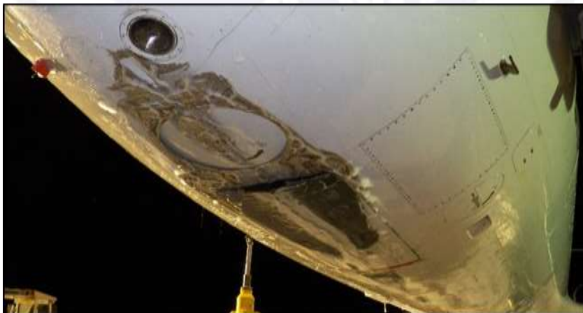
Figure 15 - Partially open landing gear doors.
