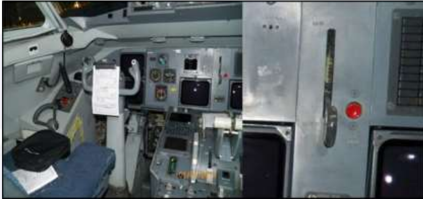
Figure 10 - Landing gear lever in the down position, LG DOWN.
