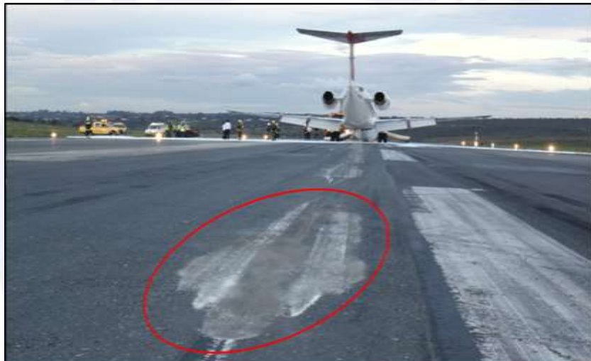
Figure 9 - Mark of the first fuselage impact.
