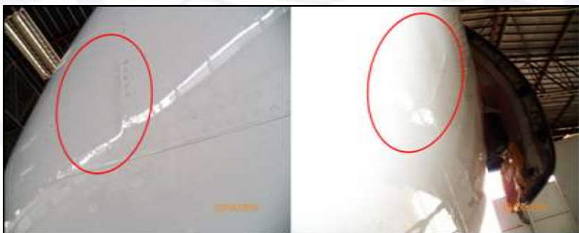
Figure 3 - Detail of the deformation in the coating and deformed rivets.
