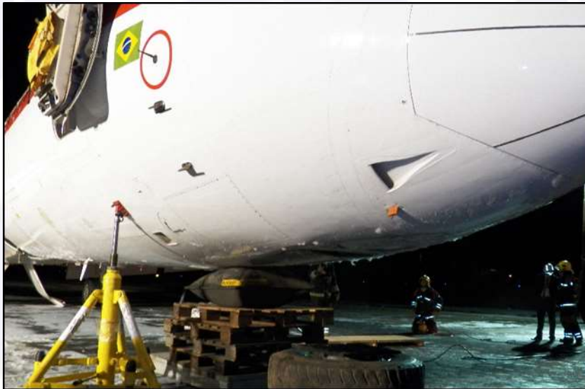
Figure 14 - Aircraft lifted by platforms, inflatables and jacks.
