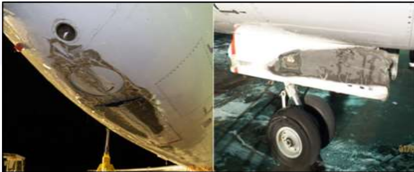
Figure 2 - Detail of the damage after lifting the aircraft and lowering the nose landing gear.
