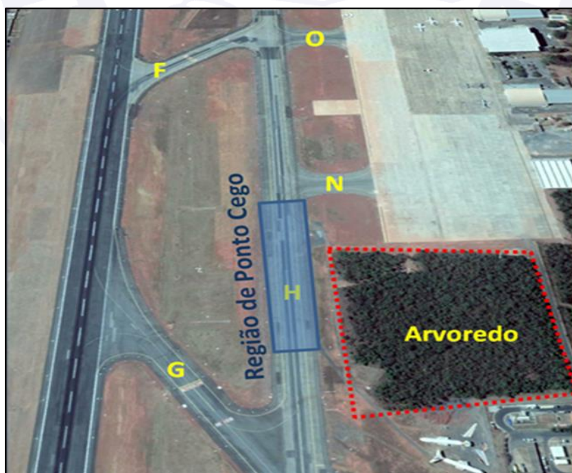
Figure 4 - Blind spot region in TWY "H" due to trees in the TWR line of sight.
