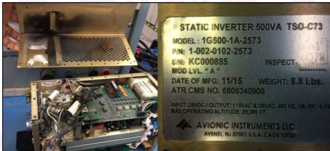
Figure 2 - Static Inverter immediately after the opening of the enclosure.
